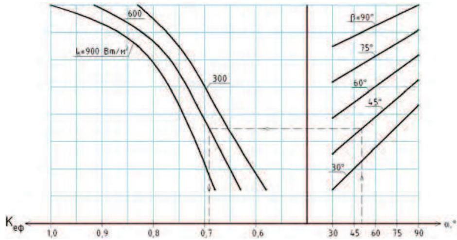
Fig. 2. Nomogram. The dependence of the efficiency of solar  $\alpha, \beta$  and  $I_B$
