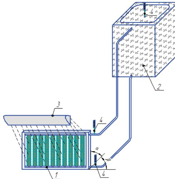
Fig. 1. Scheme of the experimental unit: 1 - solar roof, 2 - accumulator box, 3 - source of radiation, 4 - mercury thermometer
