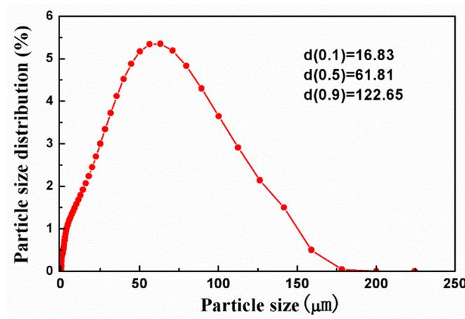
Fig. 2. The particle size distribution of collophanite
