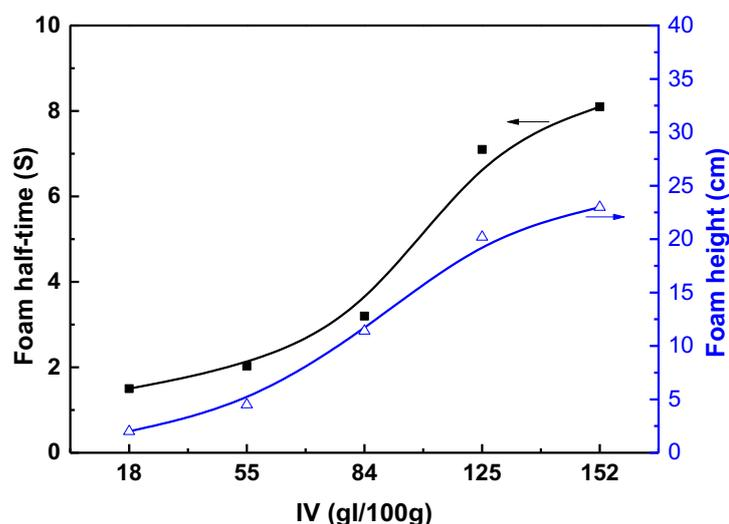
Fig. 8. The foaming ability of different sodium fatty acids, pH=10,  $C_{\text{sodium fatty acid}}=2 \times 10^{-4}$  M, 25°C
