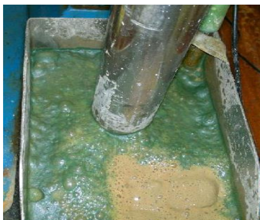
Fig. 3. A view of malachite concentrate in the second stage of sulphidisation-flotation
