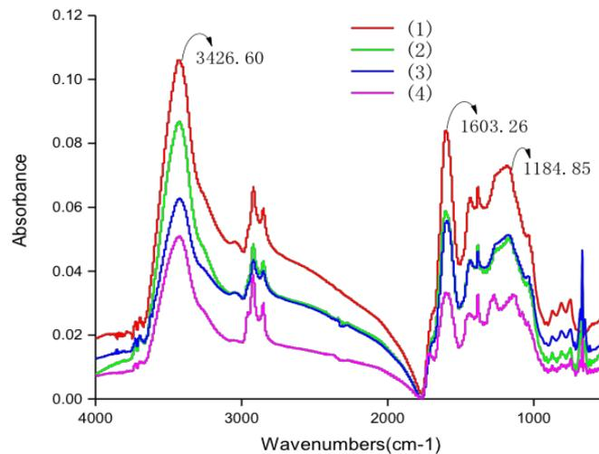
Fig. 7. FTIR spectrums of low-rank coal before and after conditioning with collectors: (1) original ultra-low ash coal, (2) ultra-low ash coal conditioned with dodecane, (3) ultra-low ash coal conditioned with n-valeraldehyde, (4) ultra-low ash coal conditioned with a mixture of n-valeraldehyde and dodecane
