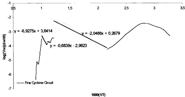
Fig. 5.  $\log(1/w)(dw/dt)$  vs  $1000(1/T)$  curve of fine circuit cyclone underflow and the combustion regions
