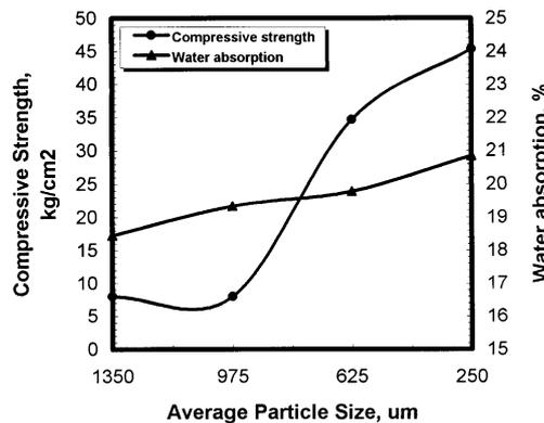
Fig. 3. Effect of particle size of sand on physical and mechanical properties of bricks
