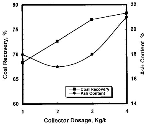
Fig. 1. Effect of collector dosage on the removal of coal fines from filter cake
