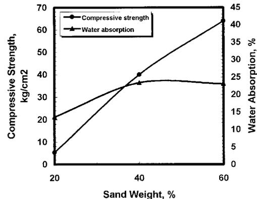
Fig. 4. Effect of weight percent of sand (for - 500 + 0  $\mu\text{m}$  size fraction) on physical and mechanical properties of bricks
