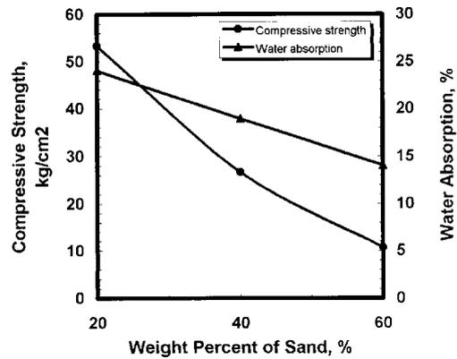
Figure 2. Effect of weight percent of sand (-1500 + 0 μm) on physical and mechanical properties of produced bricks
