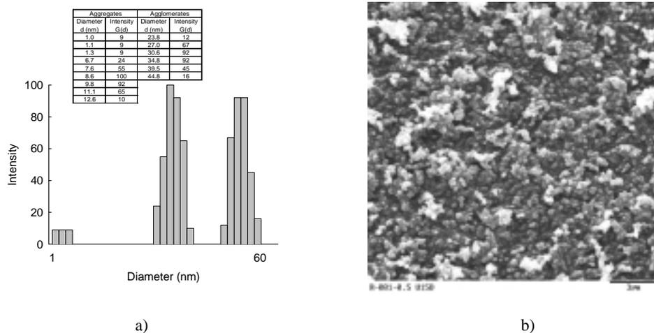
Fig. 4. a) Multimodal particle size distribution and b) SEM of TiO<sub>2</sub> modified with U-15D silane
