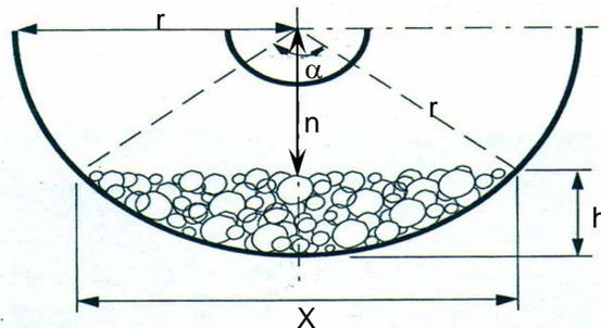
Figure 3. Cross section view of ball mill
