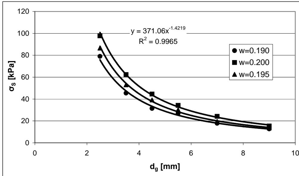
Fig. 7. Comparison of curves  $\sigma_s = f(d_g)$  for different final moisture contents of the feed ( $d_k=0.143$  mm;  $\gamma=54.79 \cdot 10^{-3}$  N/m)
