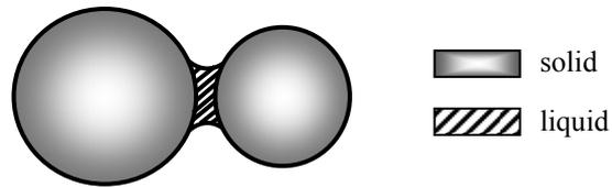
Fig. 1. Schematic of a liquid bridge between two solid surfaces
