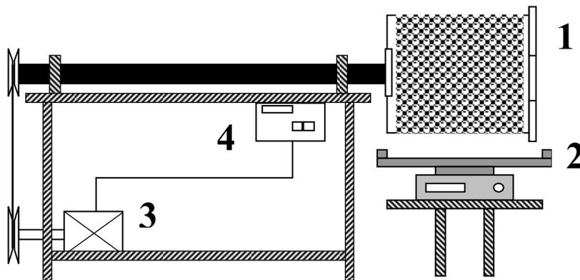
Fig. 3. Set-up for testing attrition resistance of the granulated material: 1- perforated drum, 2- balance, 3-motor, 4- inverter
