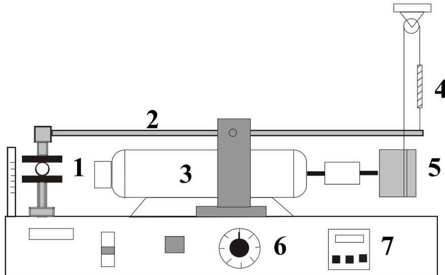
Fig. 4. Experimental set-up for testing compression strength of the granulated product: 1- compressing plates, 2- lever, 3- motor, 4- spring, 5- winding reel, 6- potentiometer, 7- torquemeter.
