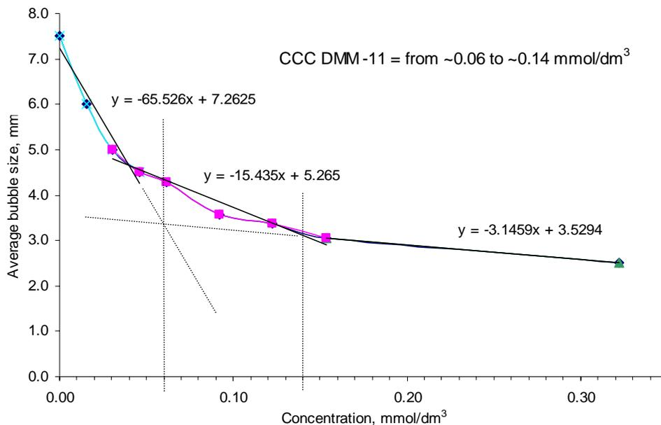
Fig. 5. Critical coalescence concentration (CCC) for DMM-11
