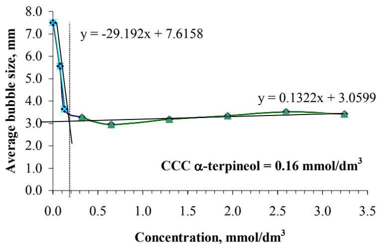
Fig. 4. Critical coalescence concentration (CCC) for  $\alpha$ -terpineol
