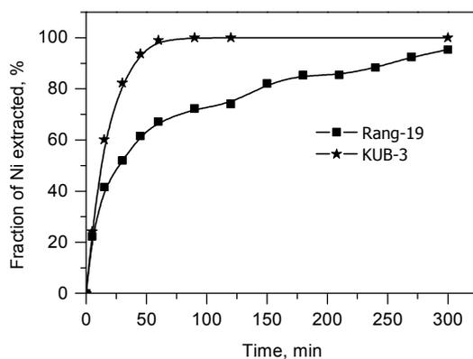
Fig. 3. Influence of leaching time on nickel extraction from the spent catalysts in 2.0 M HCl at 50°C.
