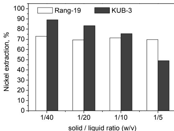
Fig. 4. Influence of the solid to liquid ratio on nickel extraction from the spent catalysts in 2.0 M HCl at 50°C after 1 hour leaching.
