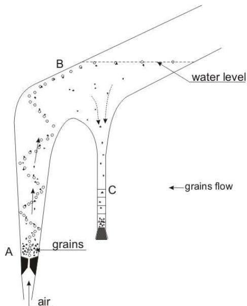
Fig. 1. Hallimond tube used in the experiments
