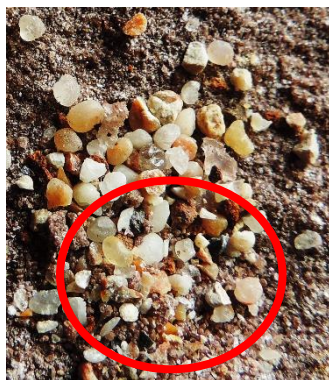
Fig. 8. Photo of the crushed sample OS 1-2 after the pressure was increased to 16 MPa. The red circle indicates the most destroyed zone
