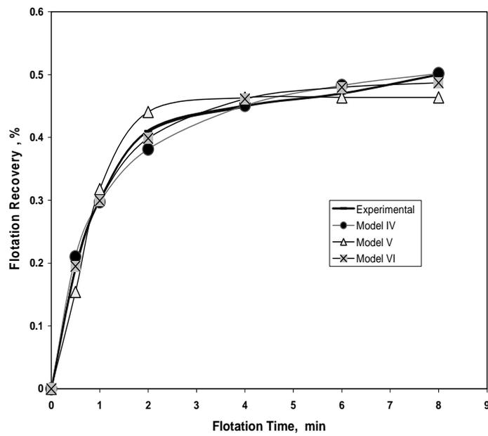
Fig. 3. Experimental and predicted flotation recovery for models IV, V, and VI at 2kg / Mg collector
