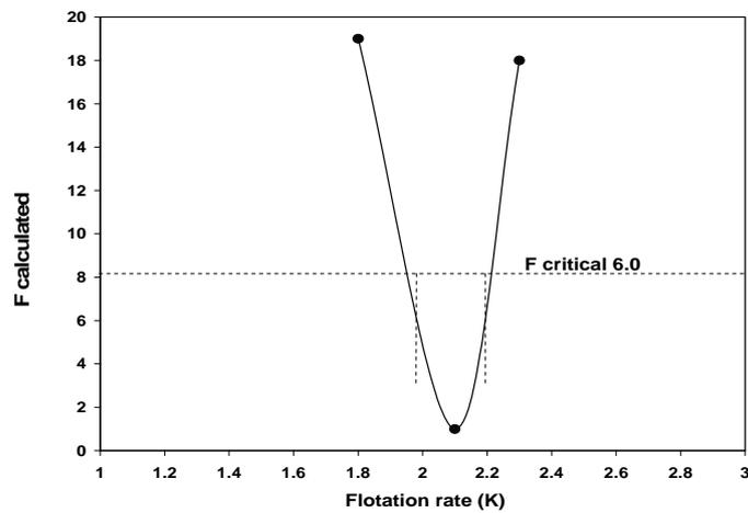
Fig. 6. Graphical determination of parameter confidence ranges for flotation rate ( $K$ ) for model II
