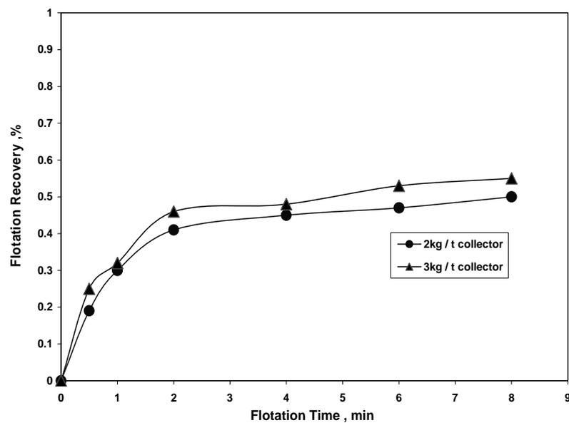
Fig. 1. Flotation response of considered feed sample at 2 kg / Mg and 3 kg / Mg collector
