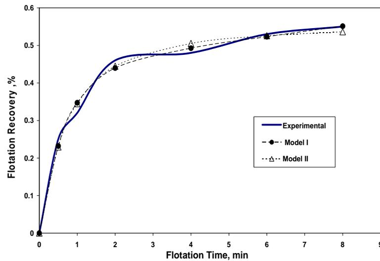
Fig. 5. Experimental and predicted flotation recovery for models I and II at 3 kg / Mg collector
