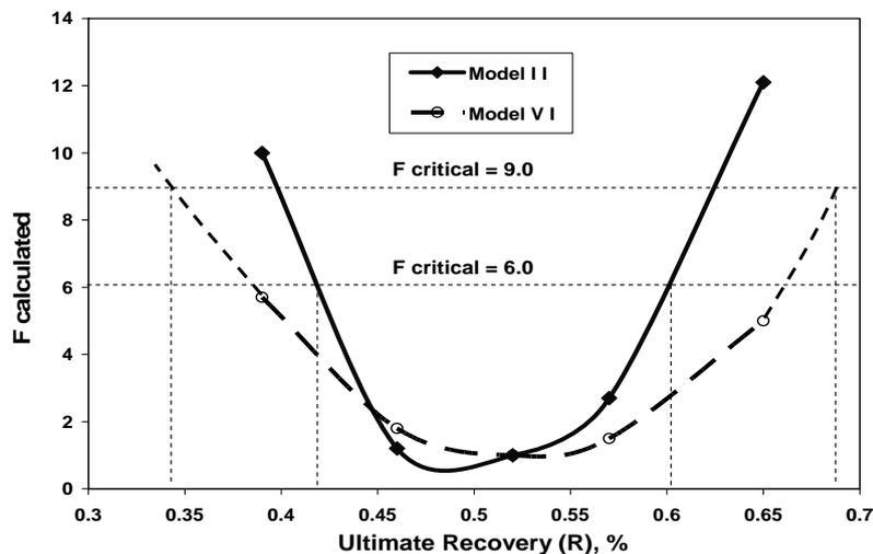
Fig. 8. Comparison of confidence ranges for ultimate recovery ( $R$ ) for models II and VI
