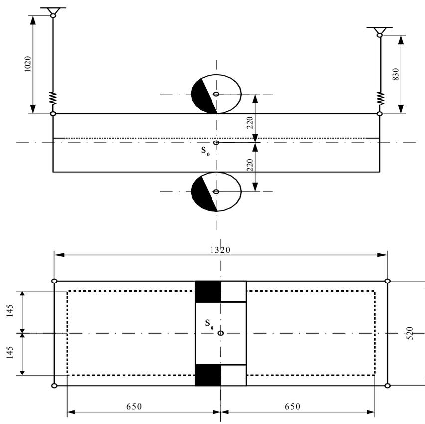
Fig. 1. The basic dimensions of the experimental screen
