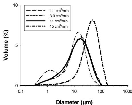
Fig. 6. Comparison of micrometric particles size distributions versus volume contribution for ZnO samples precipitated at different dosing rates of KOH solution to  $\text{Zn}(\text{CH}_3\text{COO})_2$  solution, at 20°C and at the stoichiometric ratio of the reagents
