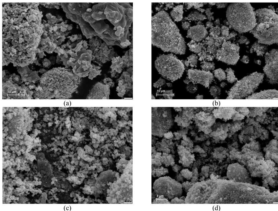
Fig. 7. SEM images of ZnO samples precipitated at different rates of dosing of KOH solution to Zn(CH<sub>3</sub>COO)<sub>2</sub> solution of (a) 1.1 cm<sup>3</sup>/min, (b) 3.0 cm<sup>3</sup>/min, (c) 11 cm<sup>3</sup>/min, (d) 15 cm<sup>3</sup>/min, at 20°C, at the stoichiometric ratio of the reagents
