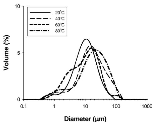
Fig. 5. Comparison of micrometric particle size distributions versus volume contribution for ZnO samples precipitated at different temperatures at a dosing rate of KOH solution to  $\text{Zn}(\text{CH}_3\text{COO})_2$  solution of  $15 \text{ cm}^3$  and at the stoichiometric ratio of the reagents
