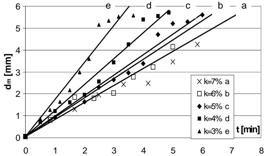
Fig. 1. The effect of wetting time (process duration) on mean particle diameter of the granulated material, for different disc filling degrees ( $D = 0.5 \text{ m}$ ,  $\alpha = 45^\circ$ )
