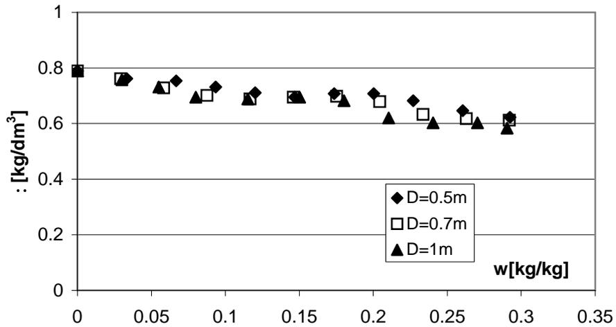
Fig. 7. Change of bulk density with an increase of bed moisture content for different disc diameters ( $k = 6\%$ ,  $\alpha = 51^\circ$ )
