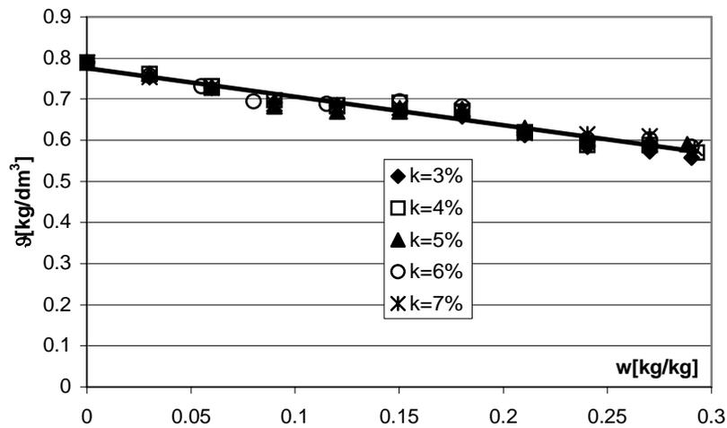
Fig. 6. Change of bulk density as a function of bed moisture content for different disc filling degrees ( $D = 1\text{ m}$ ,  $\alpha = 51^\circ$ )
