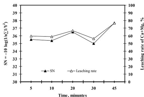
Fig. 5. The effect of dissolution time on the performance statistics for dolomite ore
