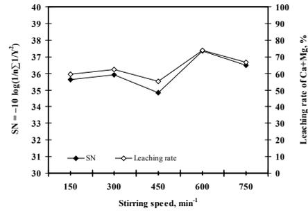
Fig. 4. The effect of stirring speed on the performance statistics for dolomite ore
