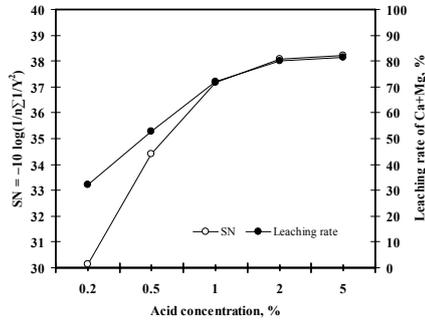
Fig. 3. The effect of acid concentration on the performance statistics for dolomite ore
