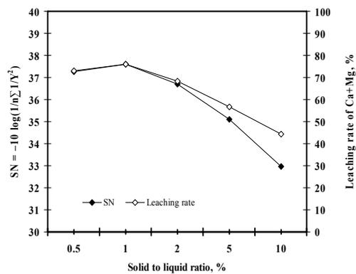
Fig. 2. The effect of solid-to-liquid ratio on the performance statistics for dolomite ore
