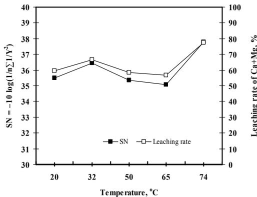
Fig. 1. The effect of leaching temperature on the performance statistics for dolomite ore
