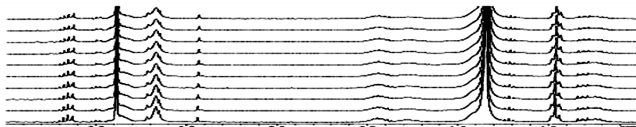
Fig. 8. The ^1\text{H} -NMR spectra of emulsions containing DTSACl in acidic conditions, sample has been tested over night with 1 hour period between spectra
