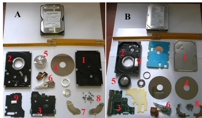
Fig. 2. Hard disks from SAMSUNG (A) and SEAGATE (B). Particular elements: 1 – top cover; 2 – mounting chassis; 3 – electronics card; 4 – platter; 5 – spindle; 6 – read/write head and head arm with ribbon cable, 7 – magnet assembly of actuator; 8 – screws, 9 – air filter
