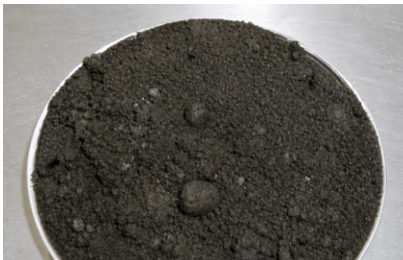
Fig. 1. Representative overall composite silicomanganese sludge sample used for physicochemical characterisation and recovery experiments
