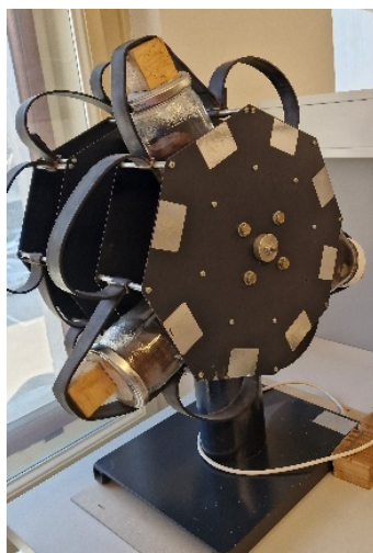
Fig. 8. Device for determining mechanical durability of briquettes (Kortnik, Anžič, 2026)
