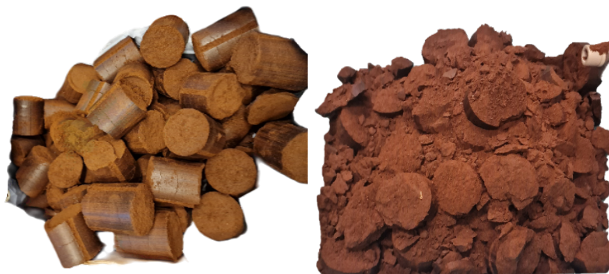
Fig. 9. Final briquettes, suitable briquettes (left) and unsuitable briquettes (right) (Kortnik, Anžič, 2026)
