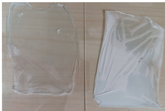
Fig. 4. Neat PU films: (a) 100 \mu\text{m} and (b) 200 \mu\text{m}
