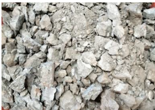
Fig. 1. Representative coarsely crushed run-of-mine (ROM) low-grade pyrolusite manganese ore collected from the Karaburun manganese deposit prior to laboratory sample preparation
