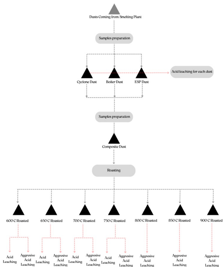
Fig. 3. Experimental flowsheet of the roasting and acid leaching tests for copper smelting dusts
