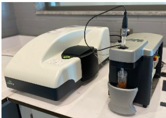
Fig. 1. Malvern Panalytical Zetasizer Ultra instrument utilized for zeta potential measurements
