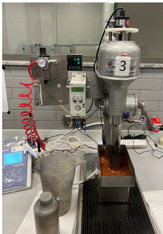
Fig. 5. Mechanical flotation machine used in flotation experiments
