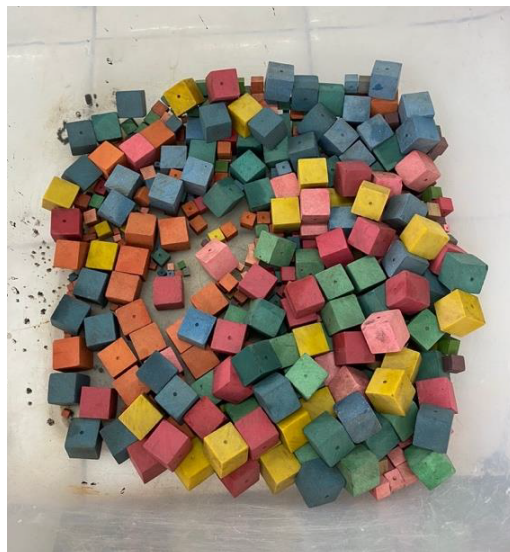
Fig. 2. Plastic density tracer cubes used to construct the partition curves. Each density class has its own colour, and 20 cubes per class were fed in each test
