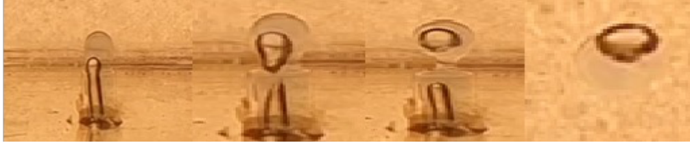
Fig. 2. Time sequence showing the formation process of a kerosene coated bubble
