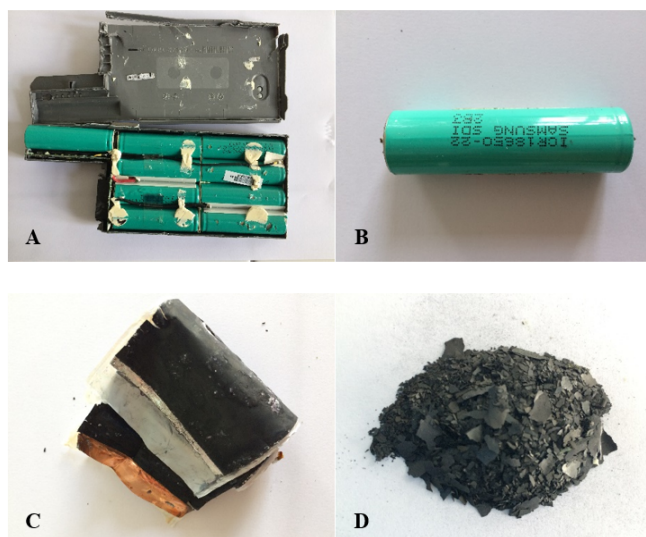
Fig. 1. Research material obtained from spent laptop LIBs after manual dismantling and manual mechanical processing; A: battery pack, B: single Li-ion cell, C: separated cell components (separator, foils and electrode powders), and D: polymetallic black mass (BM)
