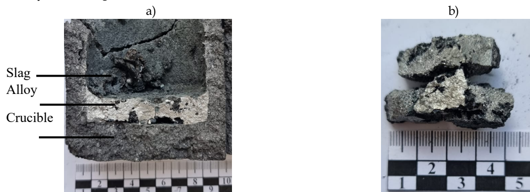
Fig. 6. Photograph of the produced ferroalloy: (a) crucible cross-section; (b) ferroalloy
