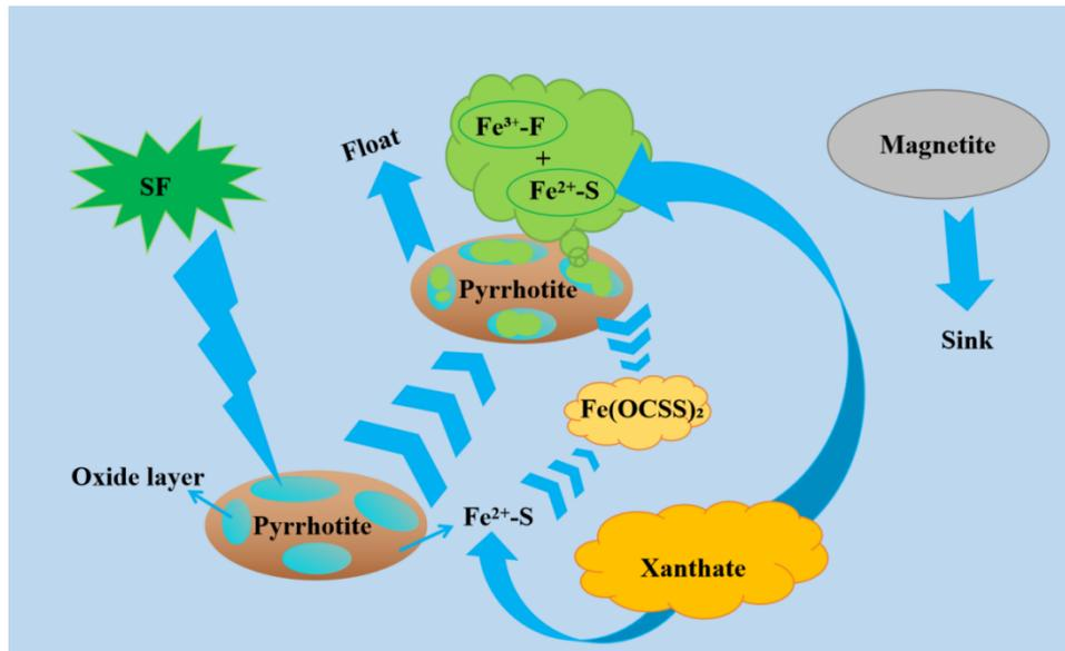
Fig. 10. Flotation model diagram of pyrrhotite and magnetite
