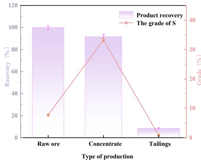
Fig. 4. Flotation test results of artificially mixed minerals
