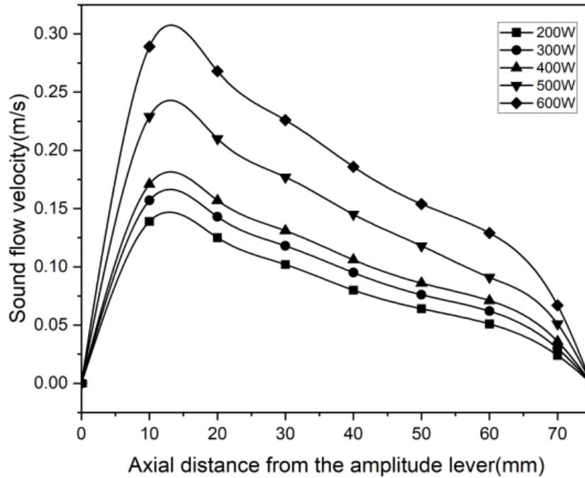
Fig. 3. Distribution of axial acoustic flow velocity in the feeding chamber under different power levels
