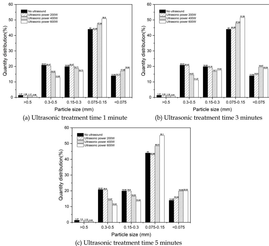
Fig. 4. Grain size distribution change of coal slime under different treatment times
