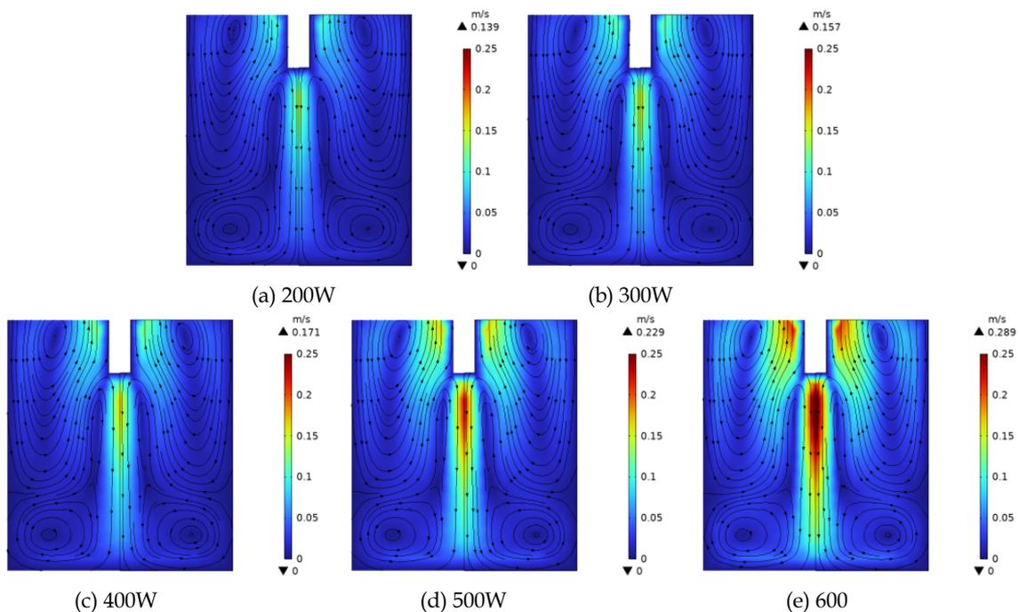
Fig. 2. Distribution of sound flow velocity under different ultrasound powers
