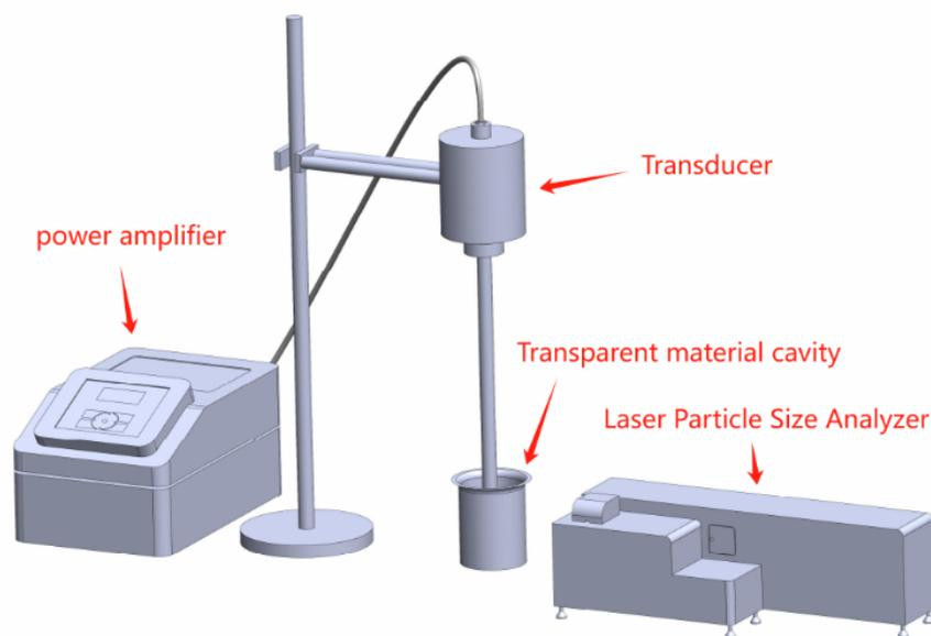
Fig. 1. Schematic diagram of experimental model
