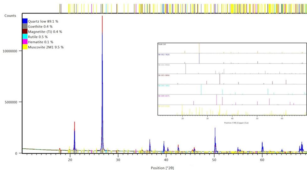
Fig. 2. XRD Rietvelt analysis of the sample
