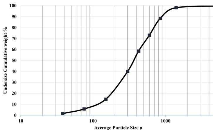
Fig. 1. Particle size distribution of the sample
