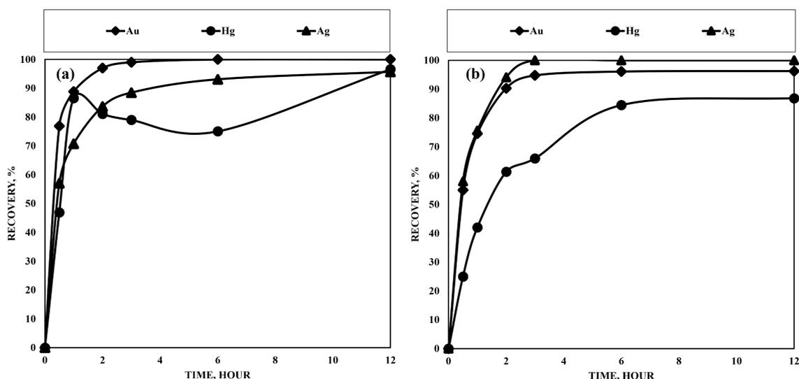
Fig. (8). Metals recovery from cyanide (a) and glycine (b) leaching solutions using AmberSep 91419 ion exchange resin, pH 10.5, 12 hours, resin/solution 2 g/l, agitation speed 200 rpm at room temperature
