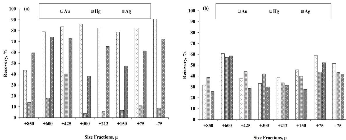
Fig. 6. Results of the original sample's size fractions cyanide leaching (a), pH 10.5, NaCN 1.5 g/l, time 24 hours, L/S 3 and agitation speed 600 rpm at room temperature. Glycine leaching (b), pH 10.5, glycine 3 g/l, potassium permanganate 3 g/l, time of 10 hours, L/S 3 and agitation speed 600 rpm at room temperature
