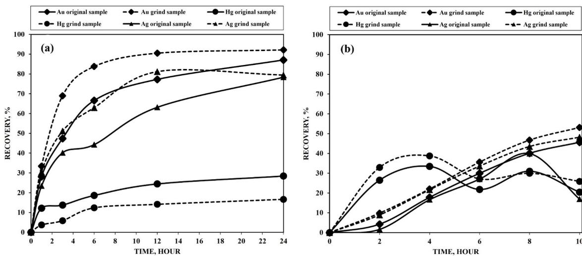
Fig. 5. Results of the original sample and grind sample cyanide leaching (a), pH 10.5, NaCN 1.5 g/l, L/S 3 and agitation speed 600 rpm at room temperature. Glycine leaching (b), pH 10.5, glycine 3 g/l, potassium permanganate 3 g/l, L/S 3 and agitation speed 600 rpm at room temperature
