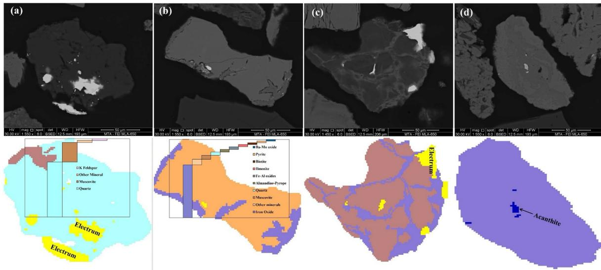
Fig. 4. SEM-BSE and classified MLA image of the light fraction (a), and heavy fraction different particles (b), (c) and (d)
