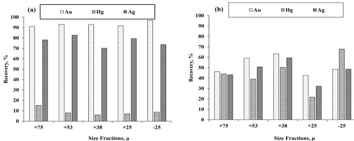
Fig. 7. Results of the grind sample's size fractions cyanide leaching (a), pH 10.5, NaCN 1.5 g/l, time 24 hours, L/S 3 and agitation speed 600 rpm at room temperature. Glycine leaching (b), pH 10.5, glycine 3 g/l, potassium permanganate 3 g/l, time of 10 hours, L/S 3 and agitation speed 600 rpm at room temperature.
