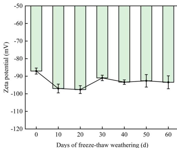
Fig. 12. Zeta potential variation of coal samples with different freeze-thaw weathering times
