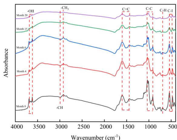
Fig. 4. FTIR of coal samples with different natural weathering times
