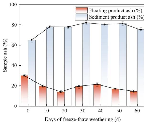
Fig. 15. Trend of ash content of integrated gangue products with different freeze-thaw weathering times
