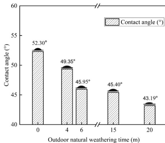
Fig. 7. Contact angle variation of coal samples with different natural weathering times
