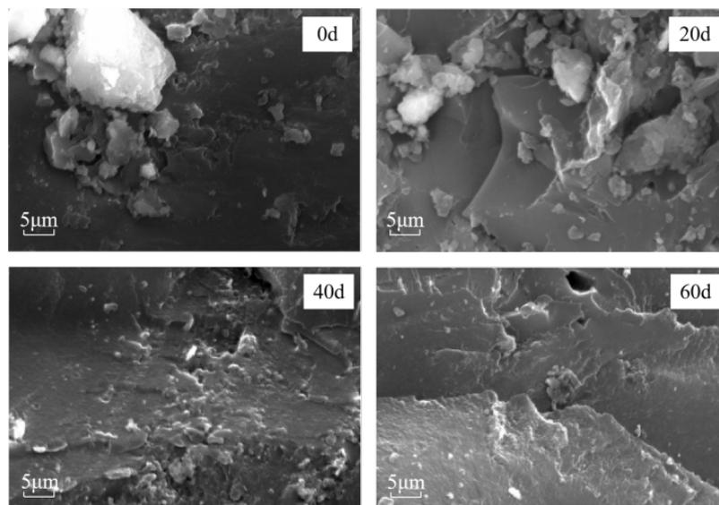
Fig. 11. Scanning electron microscopy (SEM 20,000x) of coal samples with different freeze-thaw weathering times
