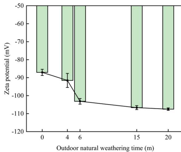
Fig. 6. Zeta potential variation of coal samples with different natural weathering times
