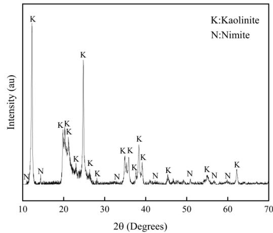
Fig. 1. XRD spectra of kaolin
