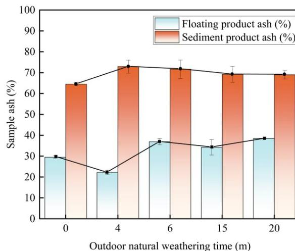
Fig. 9. Variation of ash content of coal samples with different natural weathering times
