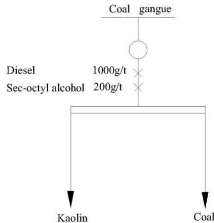
Fig. 3. Flotation test flow chart
