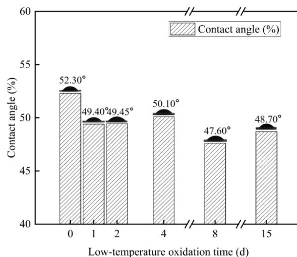
Fig. 19. Contact angle variation of coal samples with different low-temperature oxidation times
