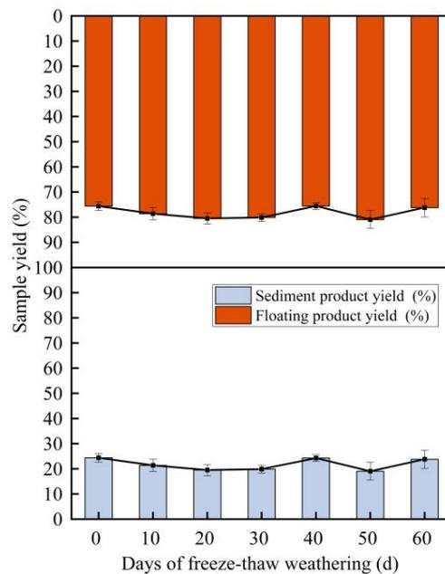
Fig. 14. Trend of coal sample yield at different freeze-thaw weathering times
