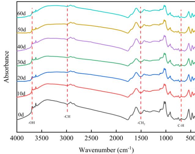
Fig. 10. FTIR of coal samples with different freeze-thaw weathering times
