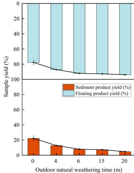
Fig. 8. Variation of yield of coal samples with different natural weathering times
