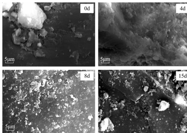
Fig. 17. Scanning electron microscopy (SEM 20,000x) of coal samples with different low-temperature oxidation times
