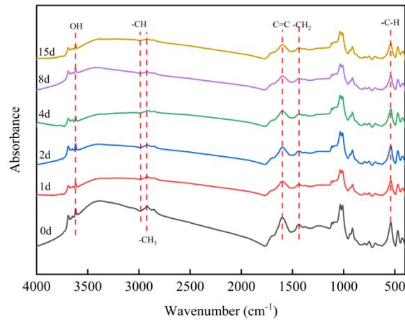
Fig. 16. FTIR of coal samples with different low-temperature oxidation times
