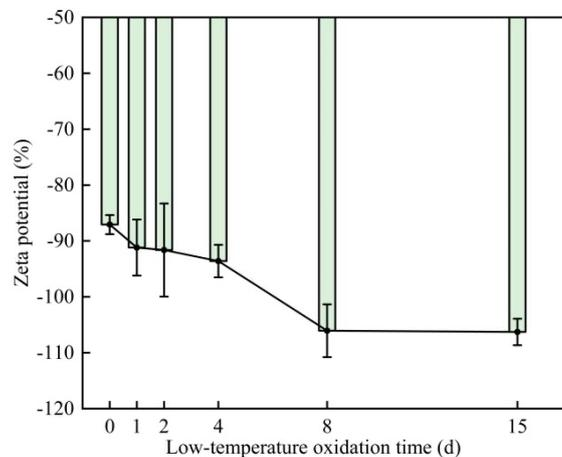
Fig. 18. Zeta potential variation of coal samples with different low-temperature oxidation times
