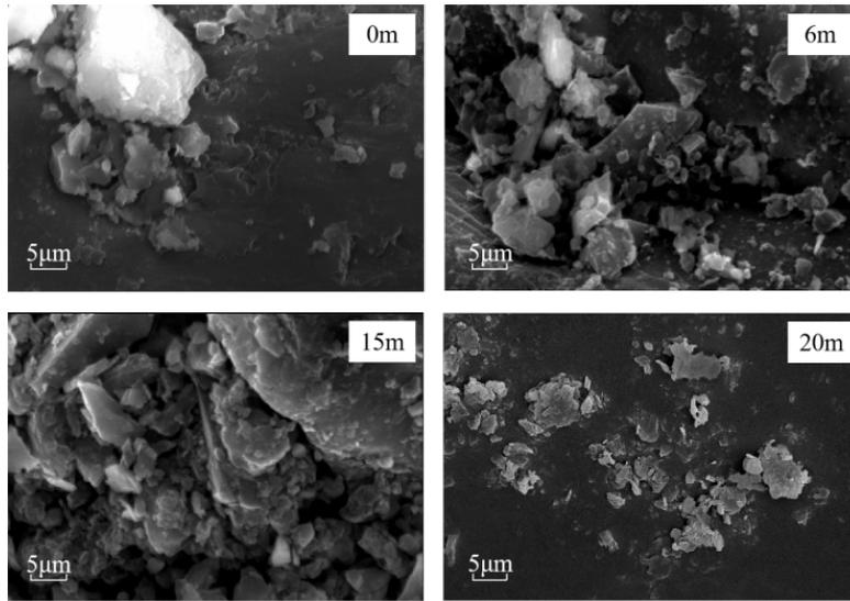
Fig. 5. Scanning electron microscopy (SEM 20,000x) of coal samples with different natural weathering times
