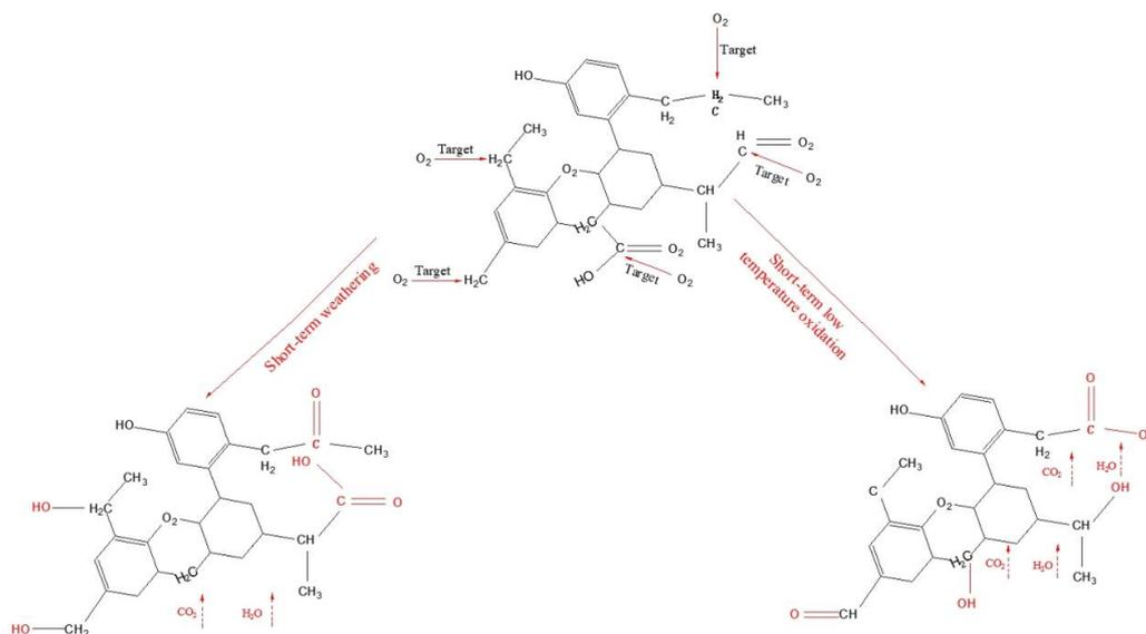
Fig. 22. Schematic diagram of weathering mechanism
