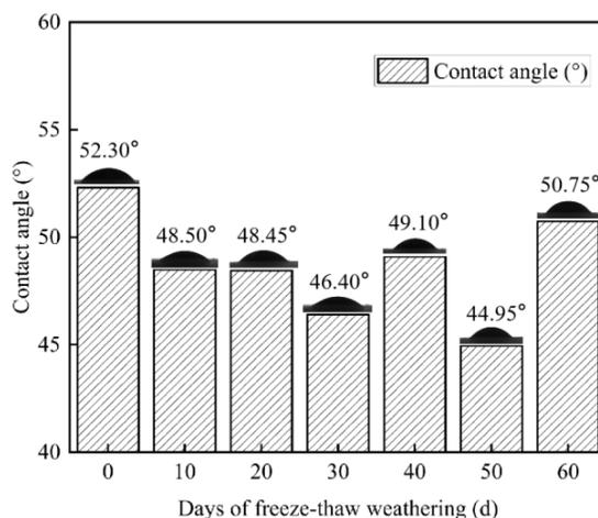
Fig. 13. Contact angle variation of coal samples with different freeze-thaw weathering times
