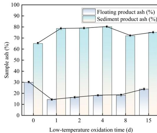
Fig. 21. Variation of ash content of coal samples with different low-temperature oxidation times
