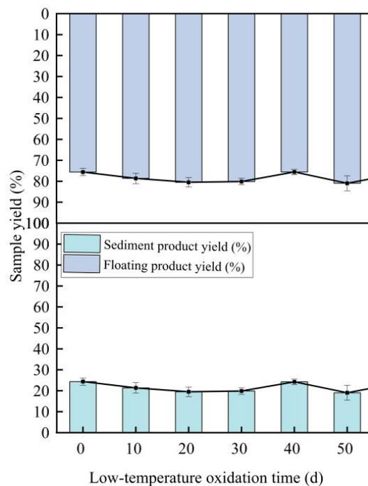
Fig. 20. Variation of yield of coal samples with different low-temperature oxidation times
