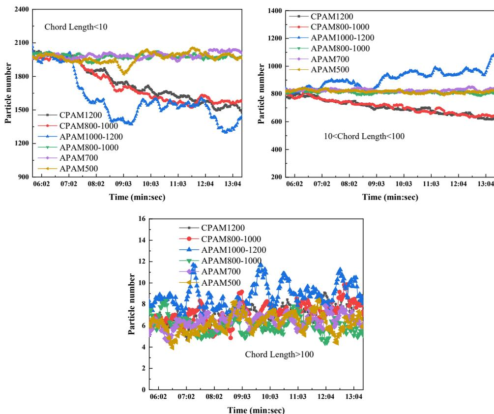
Fig. 5. Effect of polyacrylamide with different ion types and molecular weight on flocculation chord length of flocculation clean coal
