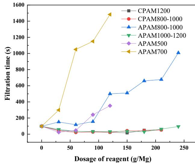
Fig. 2. Effect of ion type and molecular weight of polymer on filtration time of flotation clean coal
