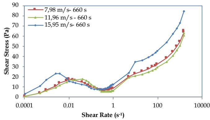
Fig. 13. Effects of 660-second mechanical activation time and peripheral speed on the flow curve
