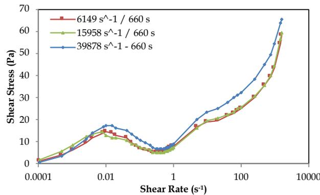
Fig. 18. Flow curve change after 660 seconds of mechanical activation at different rotor-stator designs and nominal cutting speeds
