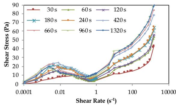
Fig. 4. Effects of mechanical activation time on the flow curve at 24000-rpm rotor speed and 15.95 m/s peripheral speed
