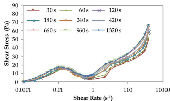
Fig. 6. Effects of mechanical activation time on the flow curve at 12000-rpm rotor speed and 7.98 m/s peripheral speed
