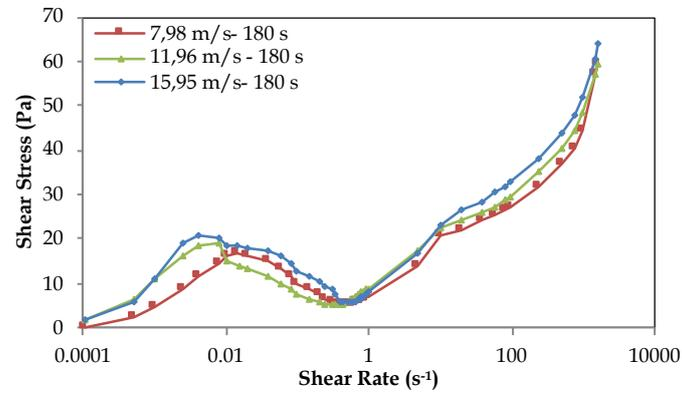
Fig. 10. Effects of 180-second mechanical activation time and peripheral speed on the flow curve
