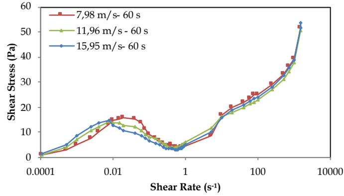
Fig. 8. Effects of 60-second mechanical activation time and peripheral speed on the flow curve
