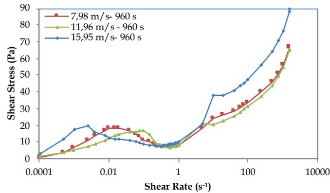
Fig. 14. Effects of 960-second mechanical activation time and peripheral speed on the flow curve
