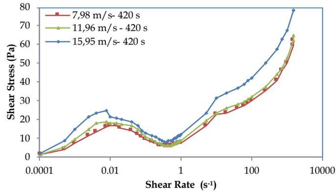
Fig. 12 Effects of 420-second mechanical activation time and peripheral speed on the flow curve
