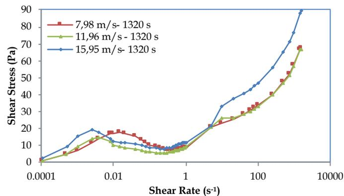
Fig. 15. Effects of 1320-second mechanical activation time and peripheral speed on the flow curve
