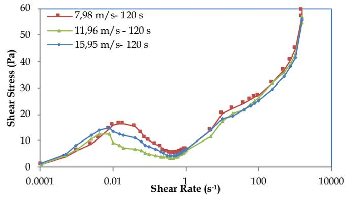
Fig. 9. Effects of 120-second mechanical activation time and peripheral speed on the flow curve
