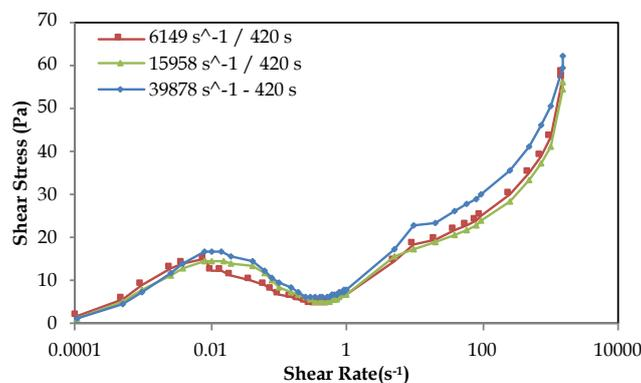
Fig.17. Flow curve change after 420 seconds of mechanical activation at different rotor-stator designs and nominal cutting speeds
