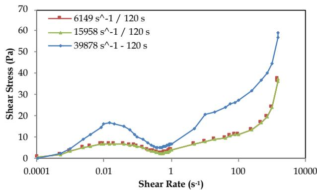
Fig. 16. Flow curve change after 120 seconds of mechanical activation at different rotor-stator designs and nominal cutting speeds
