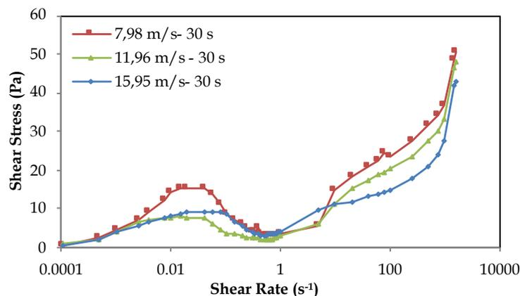
Fig. 7. Effects of 30-second mechanical activation time and peripheral speed on the flow curve
