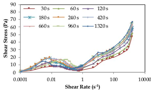
Fig. 5. Effects of mechanical activation time on the flow curve at 18000-rpm rotor speed and 11.96 m/s peripheral speed
