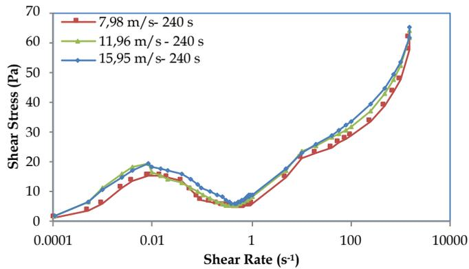
Fig. 11. Effects of 240-second mechanical activation time and peripheral speed on the flow curve
