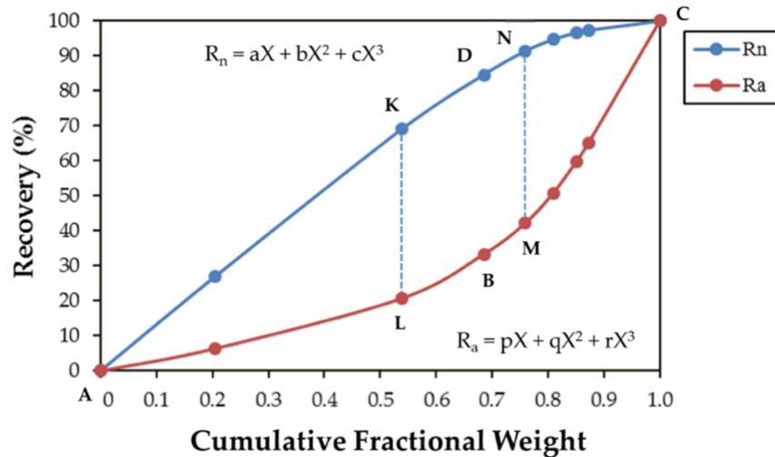
Fig. 1. Recovery curves for non-ash ( $R_n$ ) and ash-forming ( $R_a$ ) for a typical coal
