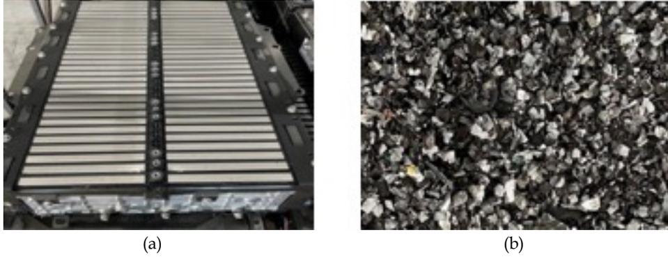
Fig. 1. The (a) battery module and (b) crushed module sample used in this study
