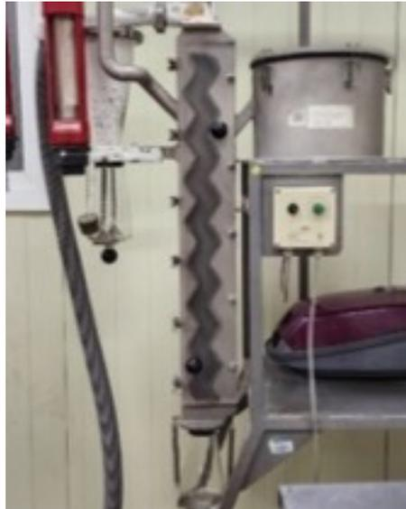
Fig. 2. Image of the zig-zag air separator utilized in the experimental setup, demonstrating the multi-stage structure for controlling particle trajectories and facilitating efficient separation
