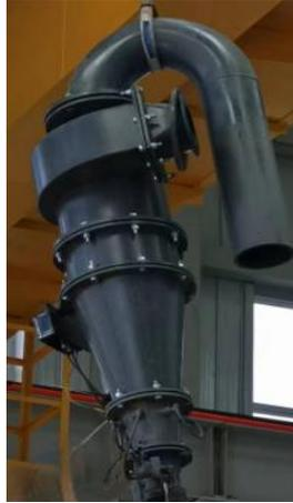
Fig. 6. Schematic diagram of water-injection hydrocyclone
