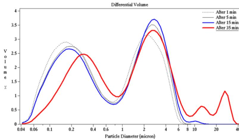
Fig. 3. CSD of phosphogypsum with 100 ppm SS at 1.502 S
