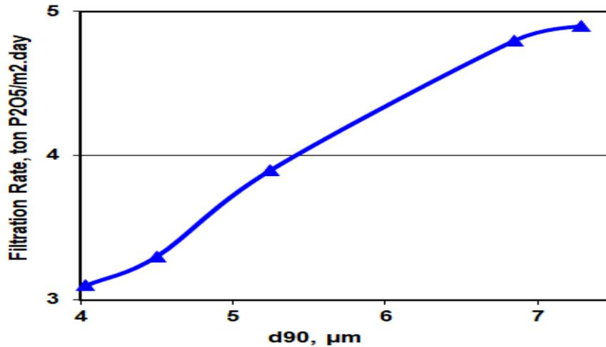
Fig. 9. Correlation between  $d_{90}$  of crystallized phosphogypsum and filtration rate ( $d_{90}$ : diameter of crystals passing 90 vol. %)
