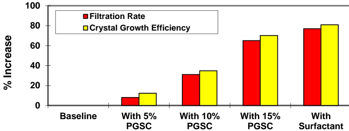
Fig. 8. % Increase in filtration rate and crystal growth efficiency of crystallized phosphogypsum with and without additives (PGSC: phosphogypsum seed crystals)
