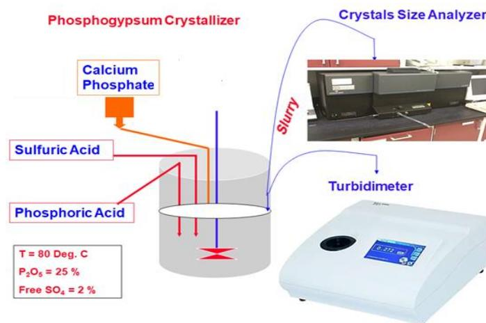
Fig. 1. Diagram indicated the experimental technique as well as turbidity and crystal size distribution (CSD) measurement apparatuses
