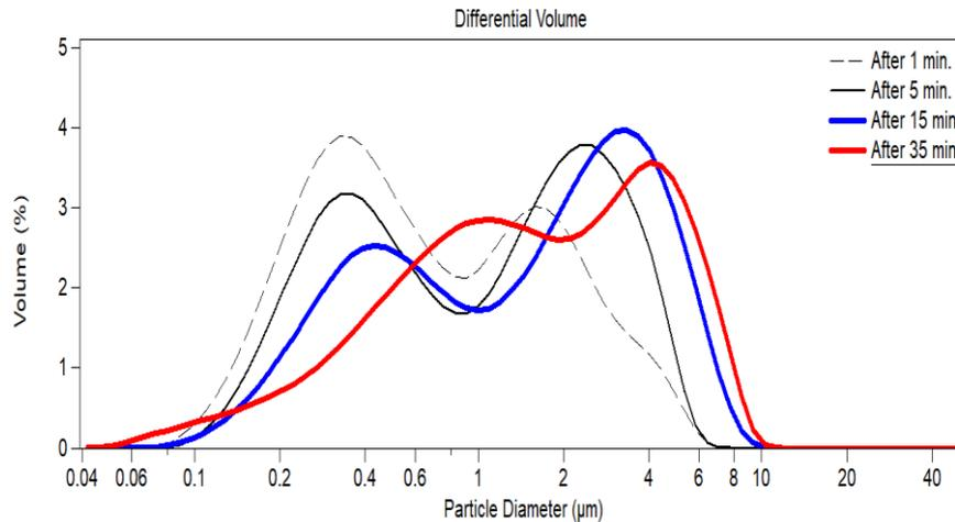
Fig. 5. CSD of phosphogypsum with 10% PGSC at 1.502 S
