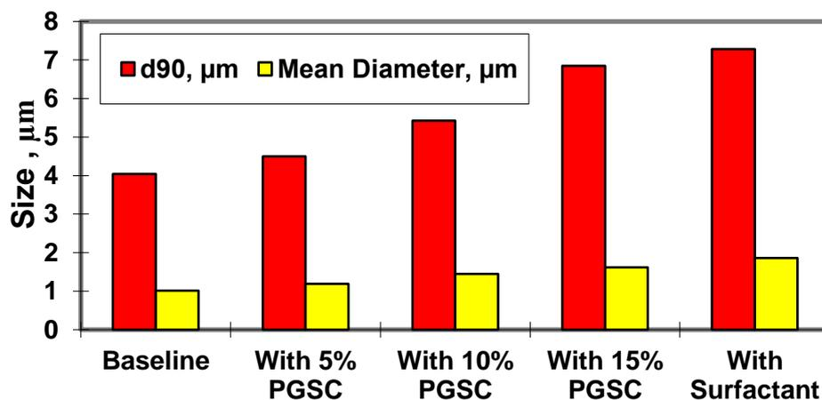
Fig. 7. Mean diameter and  $d_{90}$  of crystalized phosphogypsum with and without additives ( $d_{90}$ : diameter of crystals passing 90 vol. %, PGSC: phosphogypsum seed crystals)
