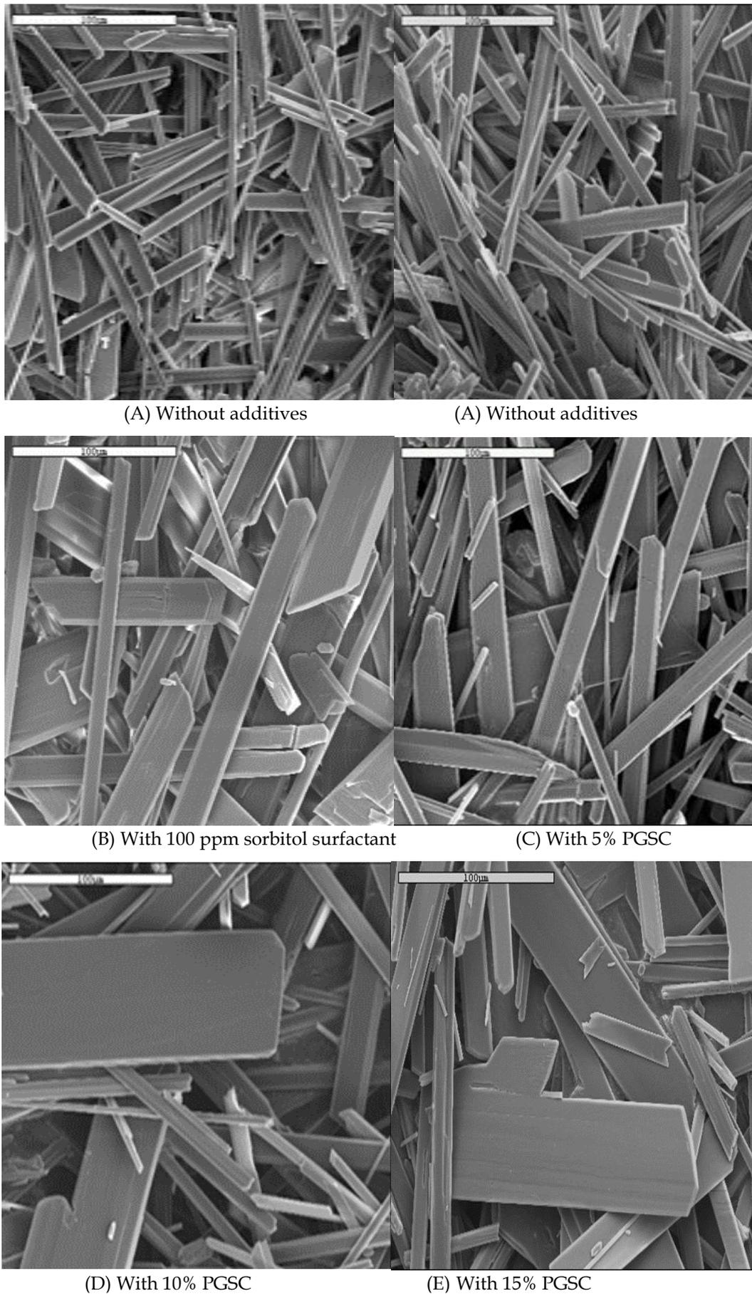
Fig. 10. Photomicrographs of phosphogypsum crystals with and without additives
