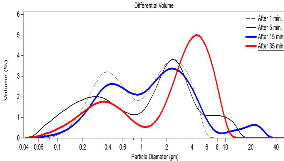
Fig. 6. CSD of phosphogypsum with 15% PGSC at 1.502 S
