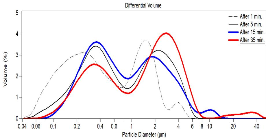
Fig. 4. CSD of phosphogypsum with 5% phosphogypsum seed crystals (PGSC) at 1.502 S
