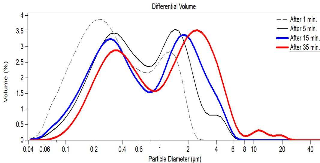
Fig. 2. Crystal size distribution (CSD) of phosphogypsum without additives at 1.502 S
