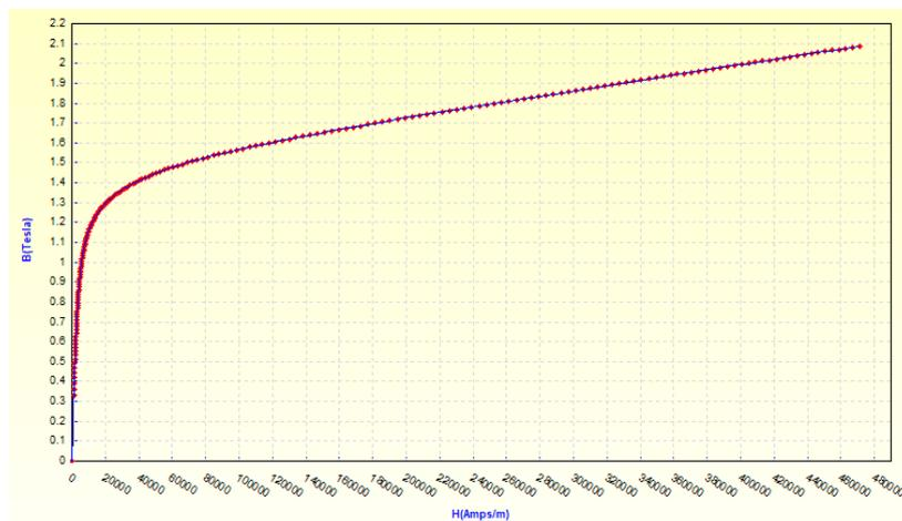
Fig. 8. B-H curve of magnetic matrix materials
