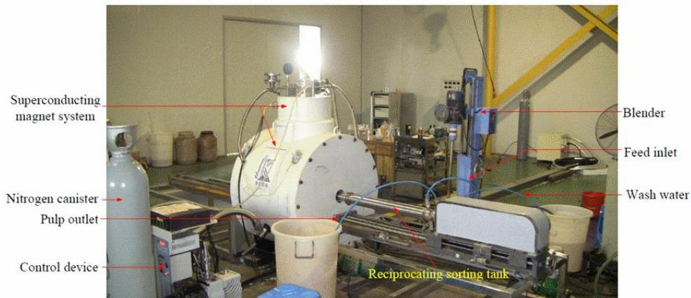
Fig. 1. A JS-6-102 pilot-scale superconducting magnetic separator
