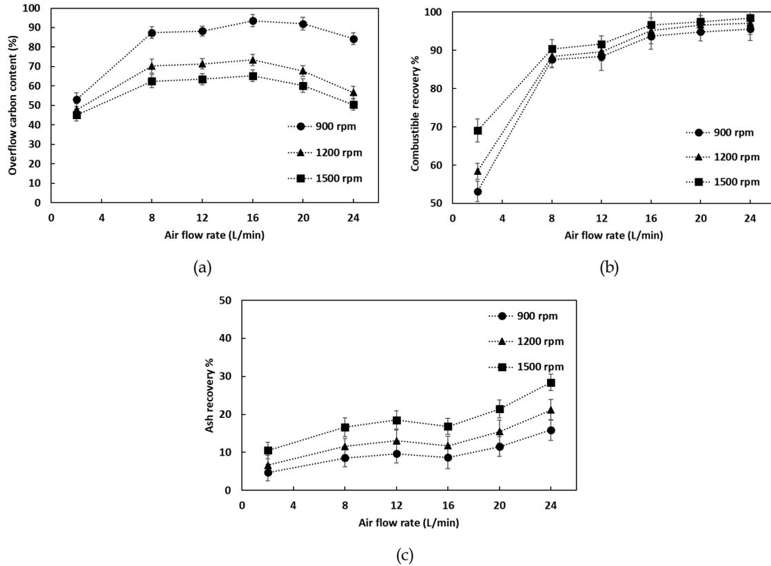
Fig. 8. Effect of (a) unburned carbon content, (b) combustible recovery, and (c) ash recovery of concentrate on agitation speed at different airflow rates
