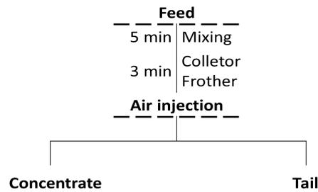
Fig. 3. Flowsheet of bottom ash flotation
