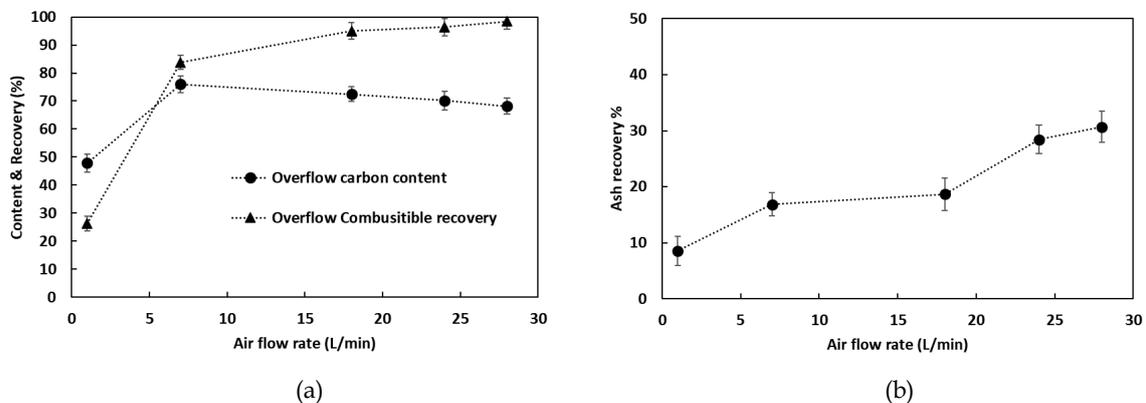
Fig. 5. Effect of (a) unburned carbon content, combustible recovery, and (b) ash recovery on airflow rate variation
