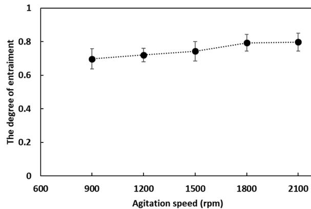
Fig. 7. Degree of entrainment of self-aerating flotation machine
