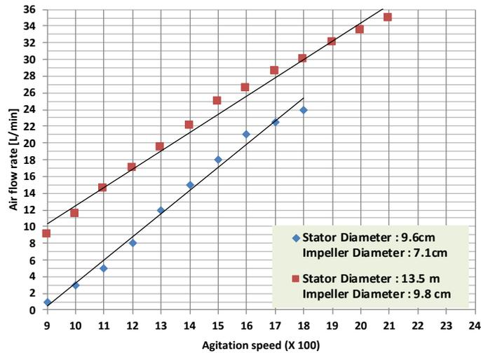
Fig. 4. Airflow rate according to the agitation speed variation
