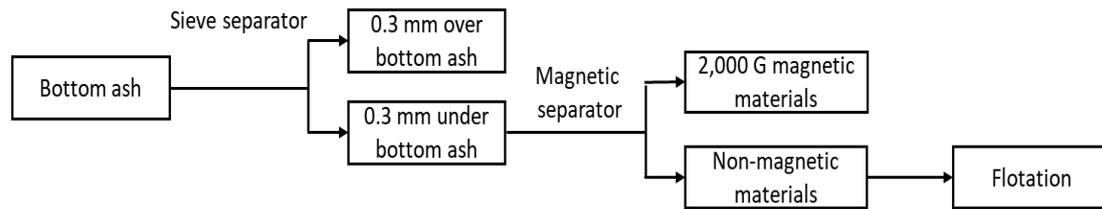
Fig. 1. Flow sheet of experiments of bottom ash
