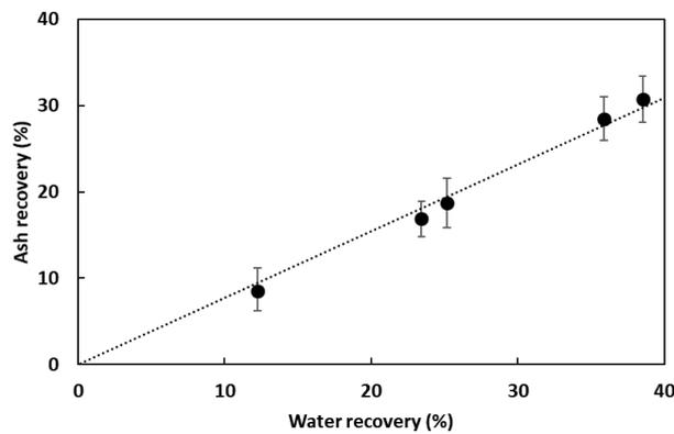
Fig. 6. Relationship between ash recovery and water recovery of concentrate.
