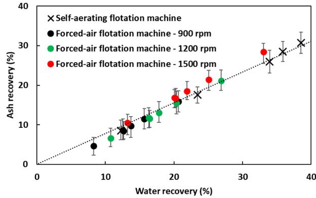
Fig. 9. Comparison of ash and water recovery between self-aerating and forced-air flotation machines
