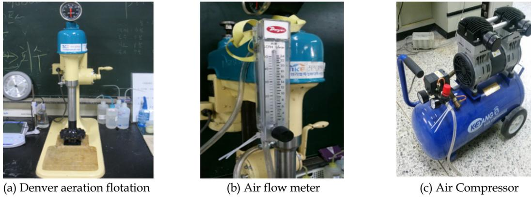
Fig. 2. (a) Self-aerating Flotation machine, (b) and (c) air injection system
