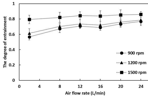
Fig. 10. Degree of entrainment of forced-air flotation machine
