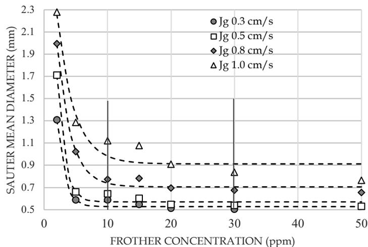
Fig. 8. Bubble size as a function of frother concentration for different gas rates
