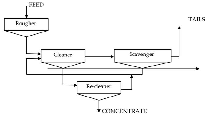
Fig. 1. Typical flotation circuit, including roughing, cleaning, and scavenging stages
