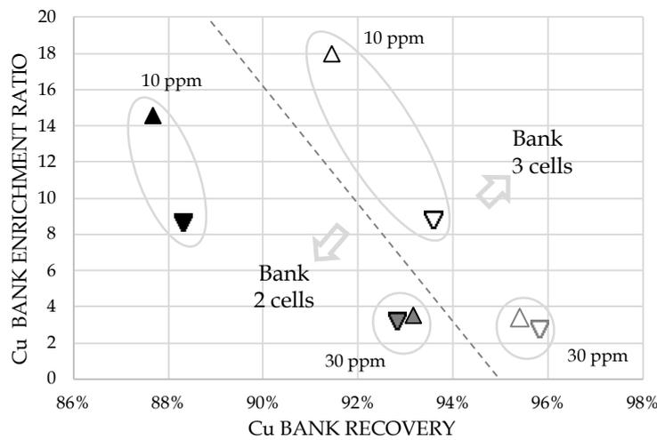
Fig. 9. Overall Cu enrichment ratio versus Cu recovery for a bank of two and three cells
