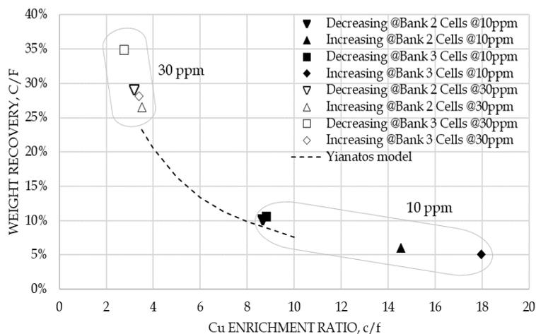
Fig. 12. Overall bank mass-pull versus copper enrichment ratio
