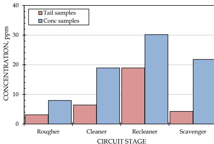
Fig. 2. Frother partitioning in a flotation circuit
