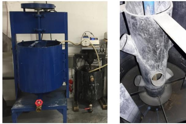
Fig. 4. (a) Conditioning tanks: 150L (blue) and 60L (black); (b) Interior view of the larger tank
