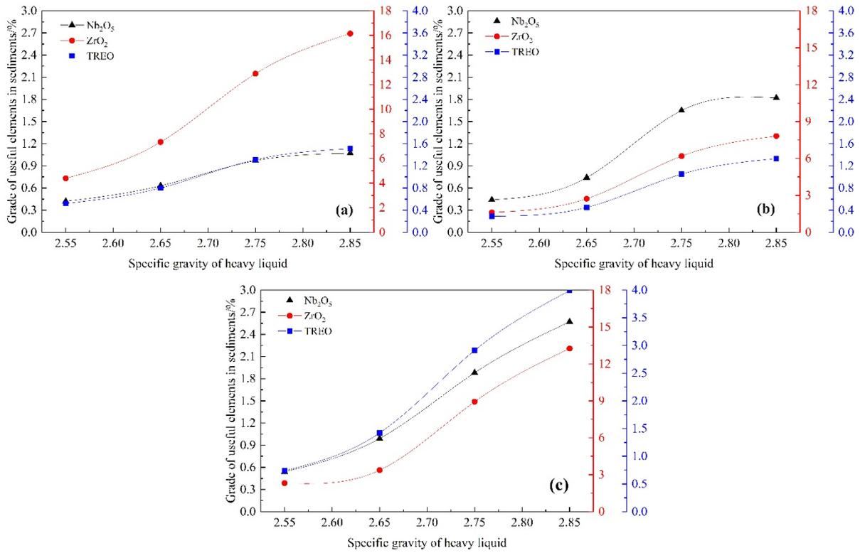
(a) -2+0.5mm size fraction; (b) -0.5+0.074mm size fraction; (c) -0.074+0.02mm size fraction
