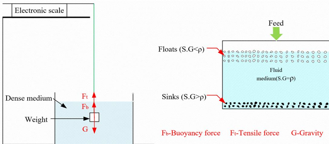
Fig. 2. Preparation of heavy liquid and experimental schematic diagram
