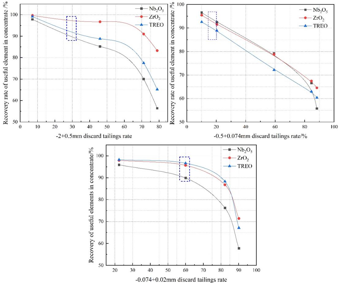
Fig. 6. Determination of tailings rates for each particle size fraction
