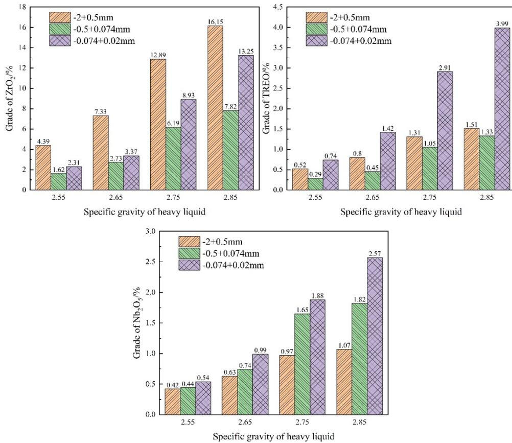
Fig. 5. Comparison of useful element grades in sinking materials at different particle sizes in the same heavy liquid
