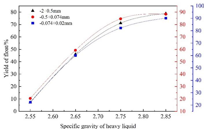
Fig. 3. The float yield of heavy liquid tests varies with specific gravity
