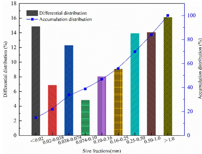
Fig. 1. Particle size distribution of -2 mm HPGR products
