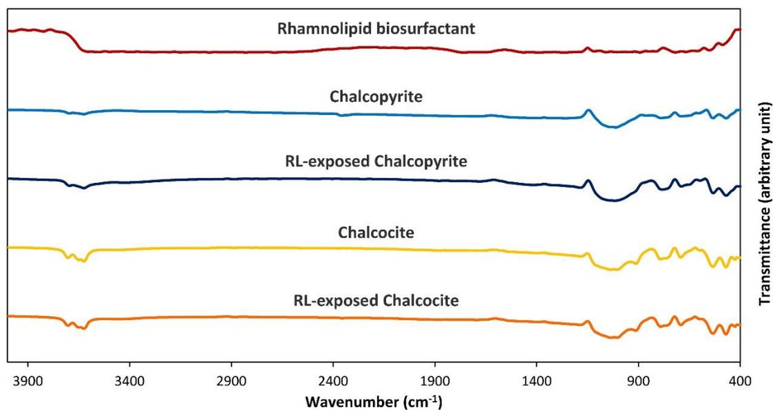
Fig. 8. FTIR spectra of pure copper minerals and rhamnolipid polluted mineral particles
