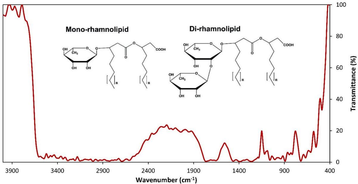
Fig. 1. FTIR spectrum of rhamnolipid biosurfactant produced from *Pseudomonas aeruginosa* strain
