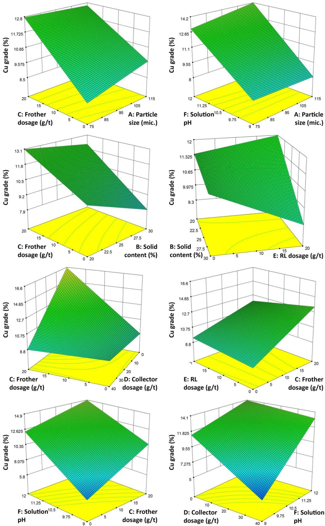
Fig. 5. Significant interaction effects among operating variables on copper grade
