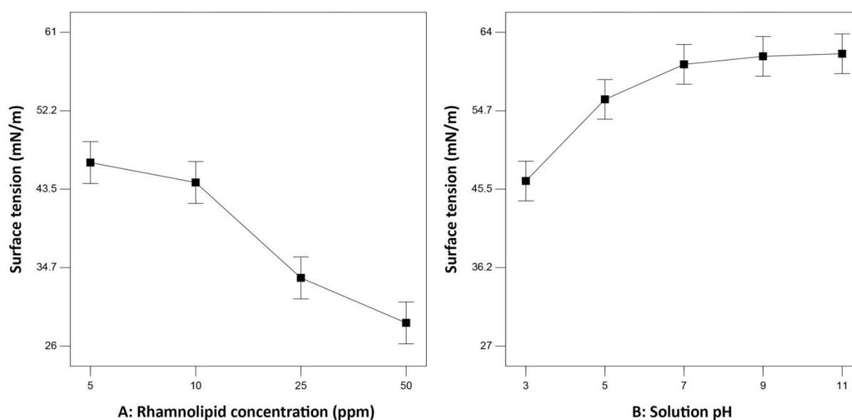
Fig. 2. Main effect plots showing the influence of selected variables on RL surface tension
