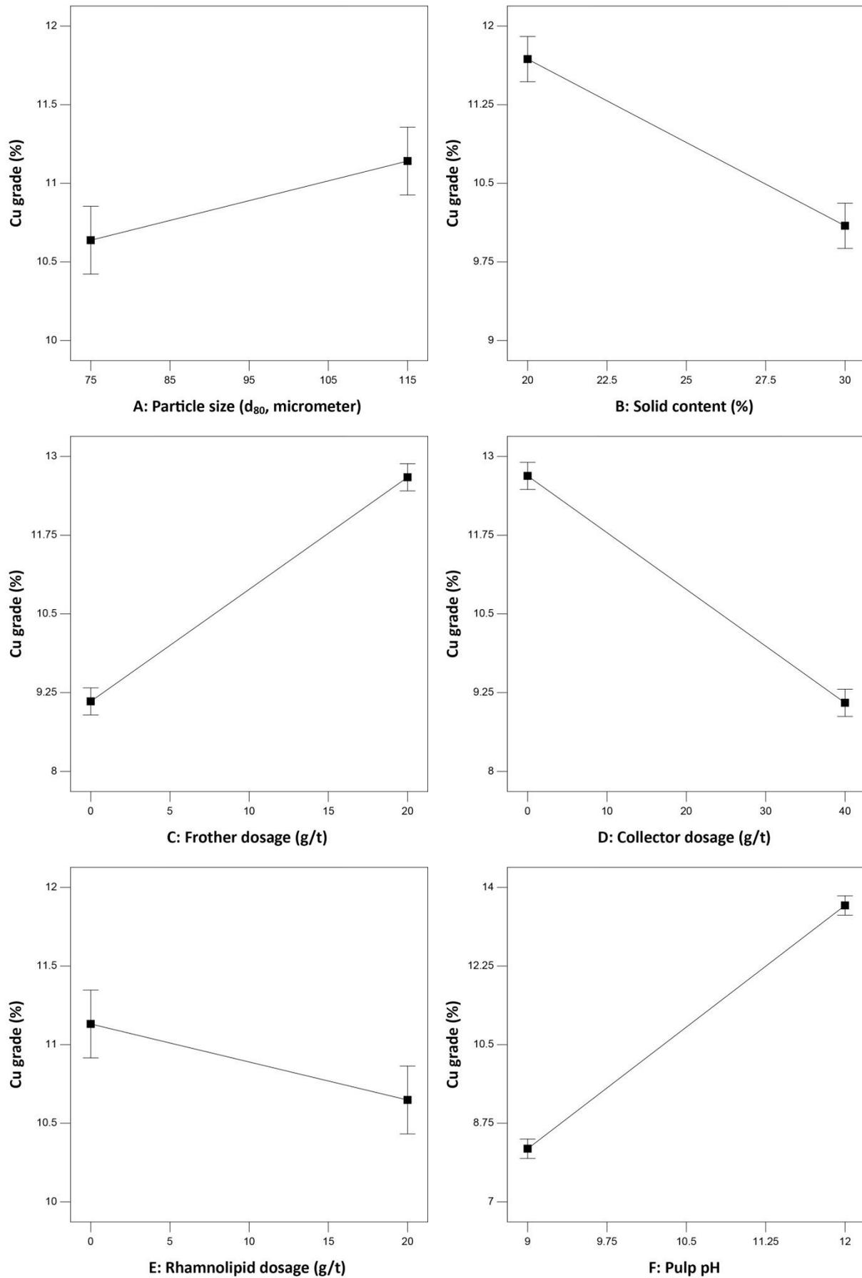
Fig. 4. Main effect plots showing the influence of operating variables on copper grade
