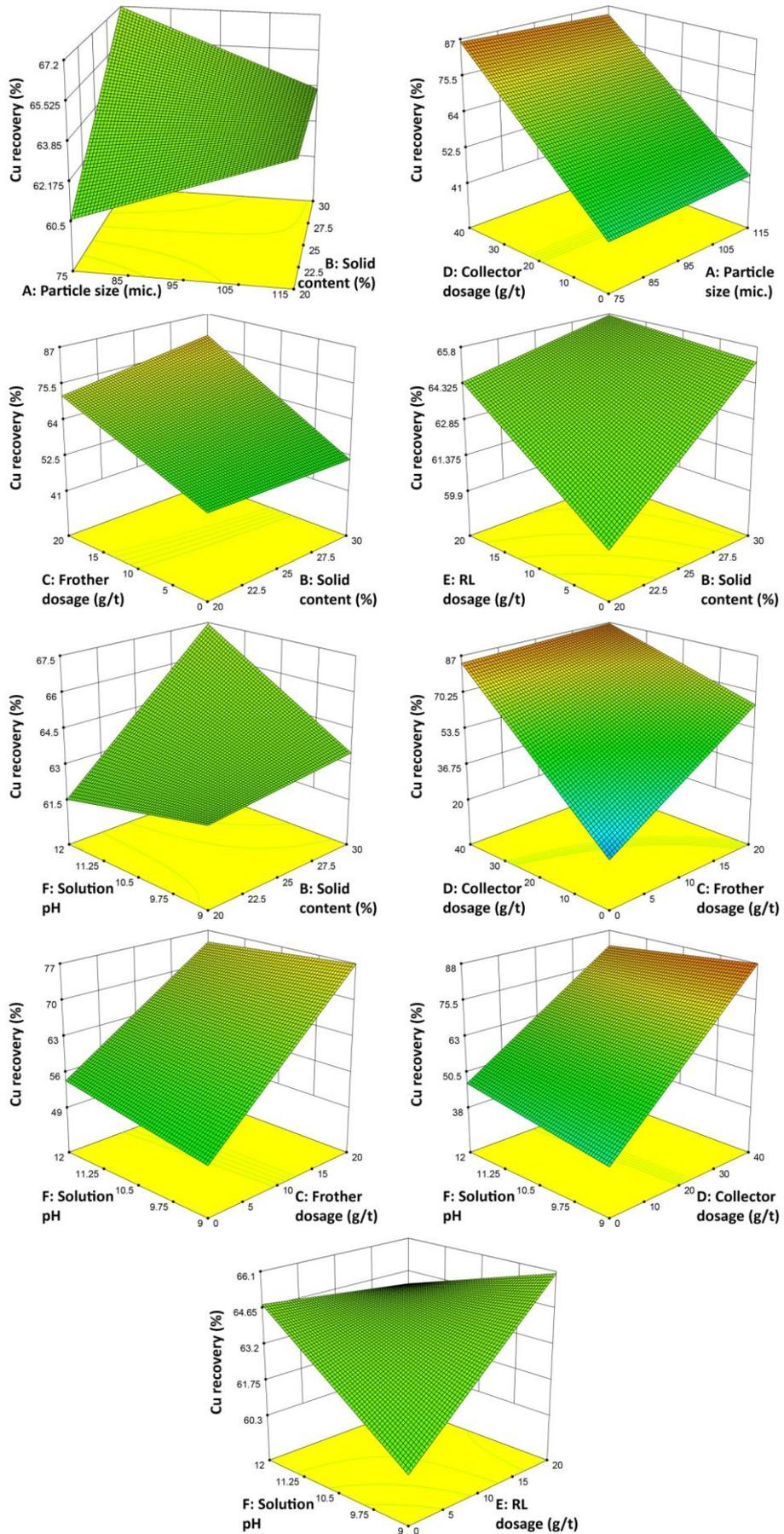
Fig. 7. Significant interaction effects among operating variables on copper recovery
