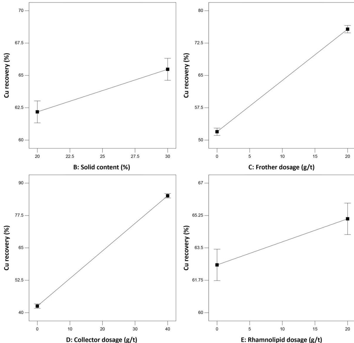
Fig. 6. Main effect plots showing the influence of operating variables on copper recovery
