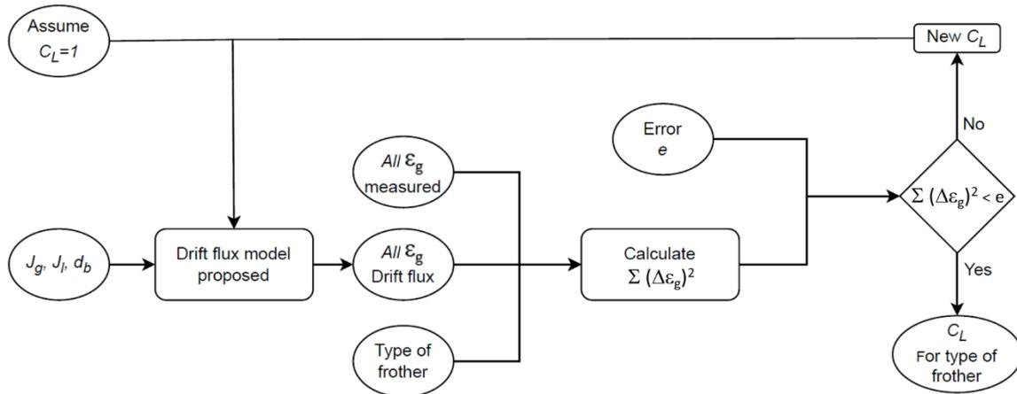
Fig. 1. Iterative model proposed for estimating parameter ( $C_L$ )
