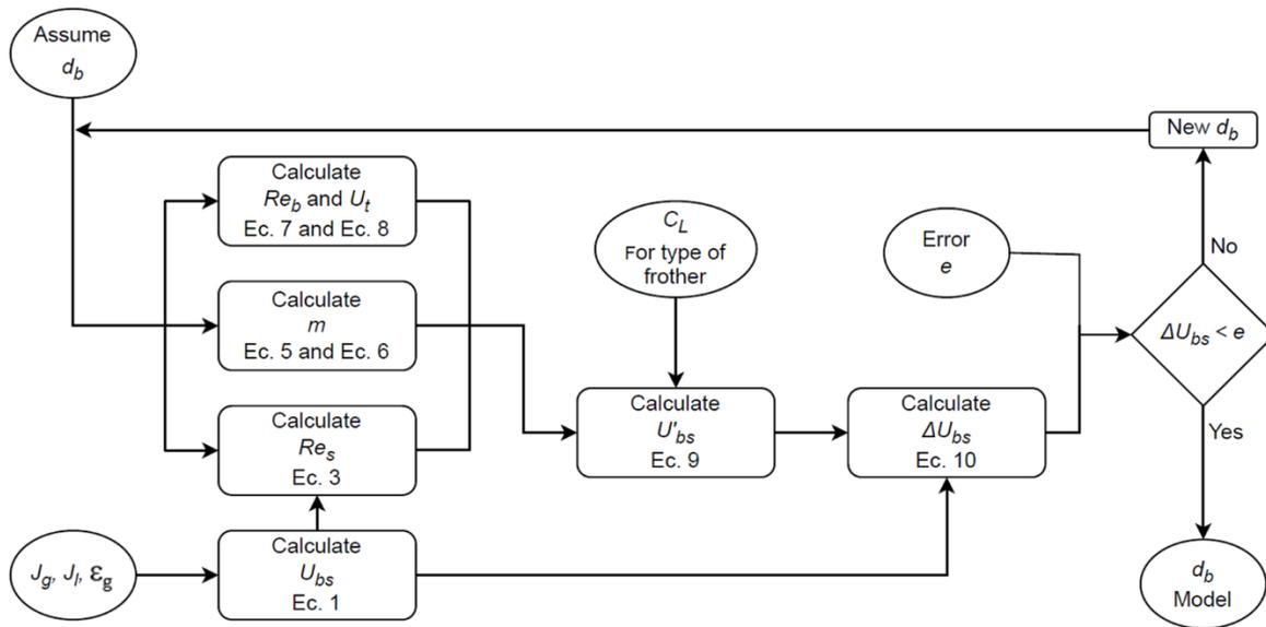
Fig. 2. Iterative model proposed for estimating bubble diameter ( $d_b$ )
