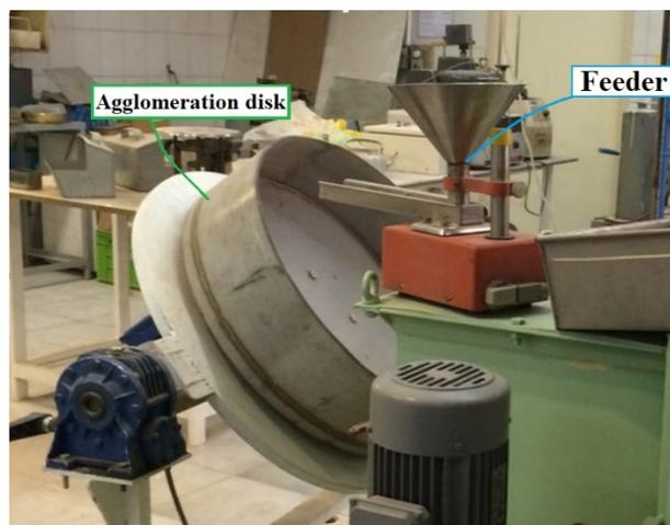
Fig. 4. Illustration of the agglomeration equipment (feeding unit and rotary drum agglomerator)
