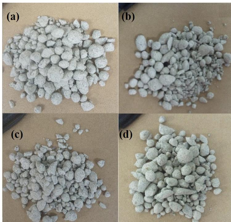
Fig. 12. Produced agglomerates with desirable quality. (a) Using Superfloc N300 before the soak test. (b) Using Superfloc N300 after the soak test. (c) Using Copolymer C2 before the soak test. (d) Using Copolymer C2 after the soak test
