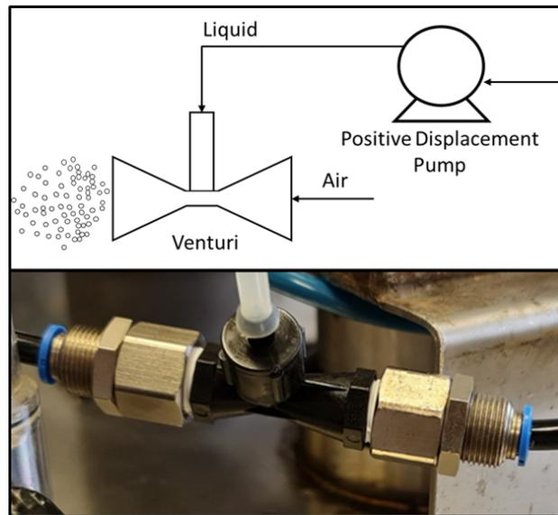
Fig. 1. Gas/Liquid venturi nozzle, with a peristaltic pump propelling the liquid
