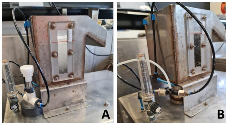
Fig. 4. Images showing the installation of (A) the nebulizer and (B) the Venturi into the airline of the flotation cell.
