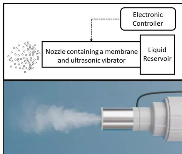
Fig. 2. Tekceleo Micronice® vibrating mesh nebulizer
