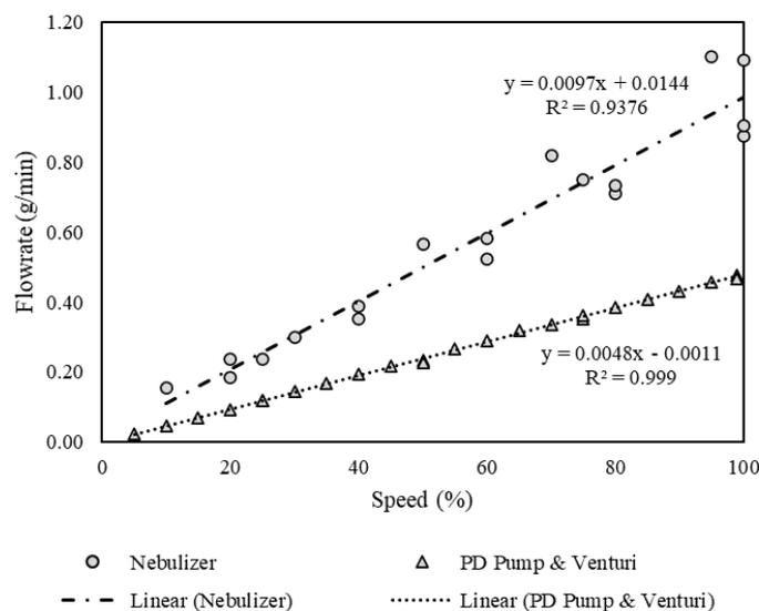
Fig. 3. Calibration curves for both the Nebulizer and the Venturi and positive displacement (PD) pump combination, as a function of both nebulizer and pump speed settings
