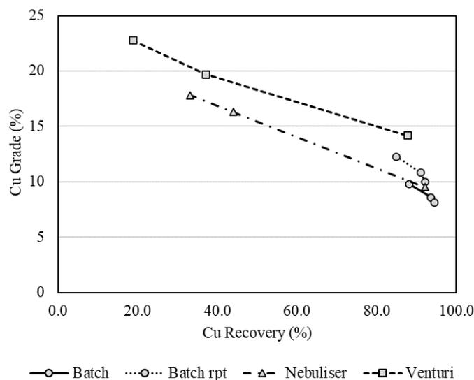
Fig. 7. Grade versus recovery curves for three different collector addition methods
