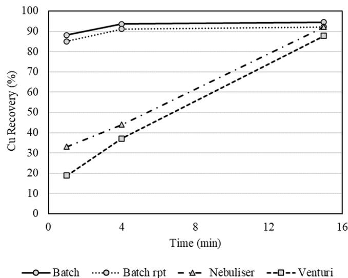
Fig. 6. Time versus recovery curves for three different collector addition methods
