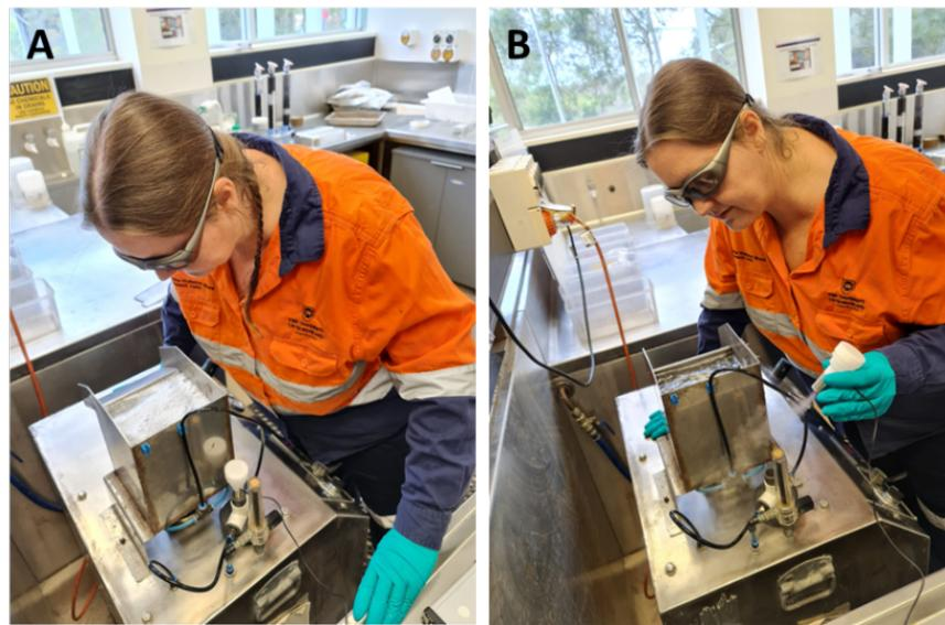
Fig. 5. Safety test using the Bitrex solution (A) nebulized into the flotation cell, (B) nebulised into the air next to the flotation cell as a control.
