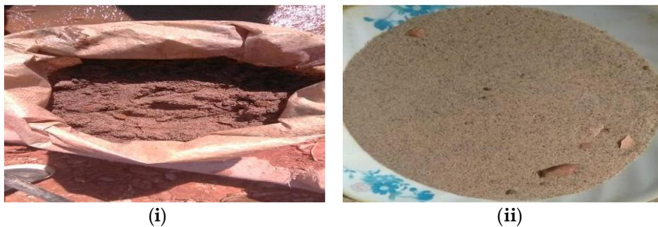
Fig. 2. Rayfield-Jos alluvial columbite mineral (i) As-received (ii) Washed and dried sample
