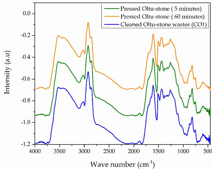
Fig. 4. FTIR spectra of cleaned Oltu-stone and pressed Oltu-stones
