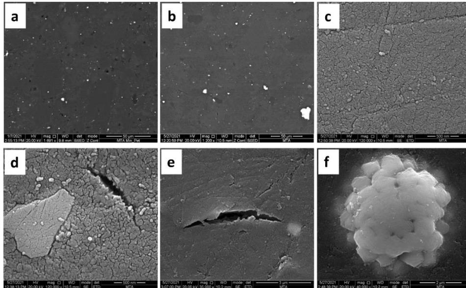
Fig. 3. SEM images of pressed Oltu-stone, a). Top surface b). Cross-sectional surface c). Nano pores d). Meso and macropores e). Macro pores. f). Framboidal pyrite filled with mobilized liptinite content
