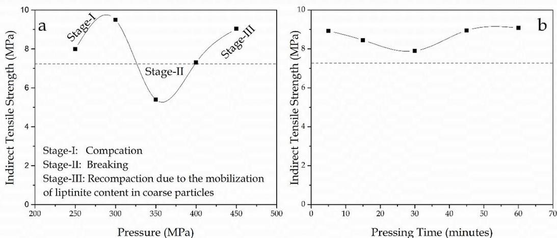
Fig. 2. Indirect tensile strength of pressed Oltu-stone at a) different pressure (MPa), with constant pressing time (1 hour) Indirect tensile strength of pressed Oltu-stone at pressing time (minute), with constant pressure (450MPa)
