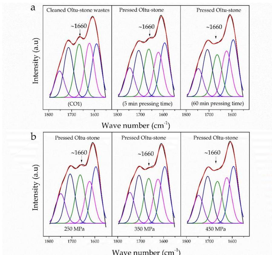
Fig. 5. a) Oxygenated group region fitted curve of figure 4. b) oxygenated group fitted curves of pressed Oltu-stone under different pressures conditions with constant time (60 minutes)
