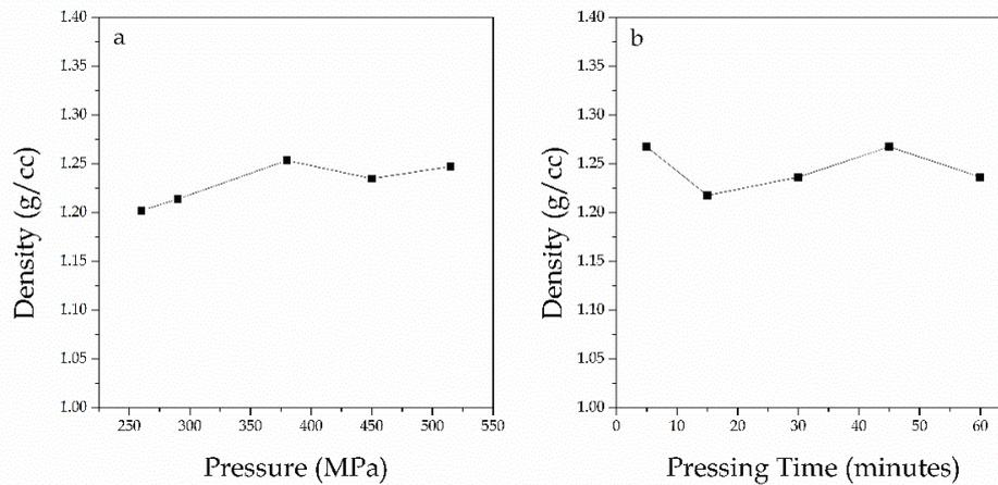
Fig. 1. Bulk density of pressed Oltu-stone a) different pressure with a constant time of one hour and b) different pressing time at 450 MPa
